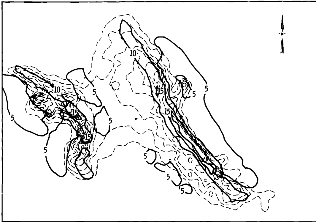
FIGURE 3.2. Wind Speed Contours at 15 m Above the Surface for Idealized Tradewind Flow Over Oahu. The free stream wind speed at 200 m was 10 m/s and the wind direction was 65°.
