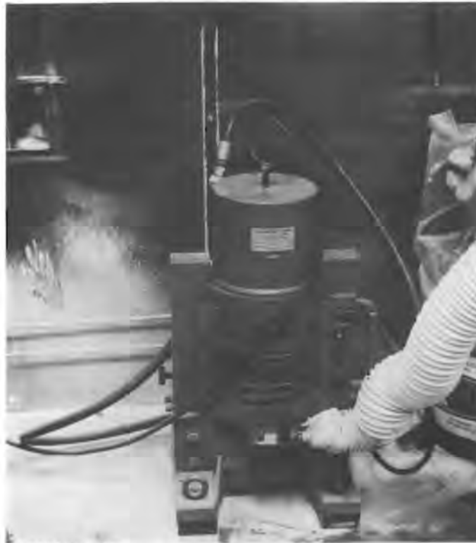
FIGURE 5.2. Double-Cut Shear Used To Section Plutonium-Contaminated Metals Prior to Decontamination by Vibratory Finishing
