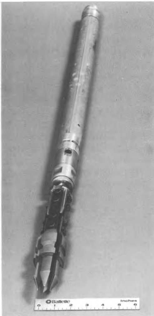
FIGURE 5.7A. Assembled Sample Recovery Device Decontaminated Using Citric Acid Bath and In Situ Electropolishing Techniques
