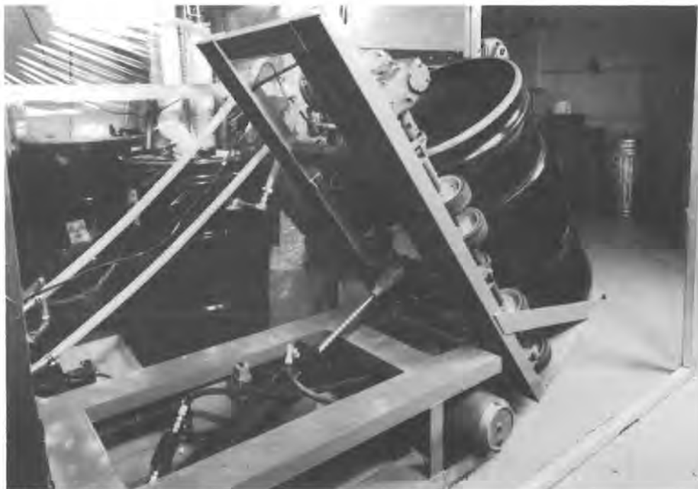
FIGURE 5.6. Apparatus Used for In-Drum Solidification of Plutonium-Contaminated Liquid Waste Using Portland Cement
