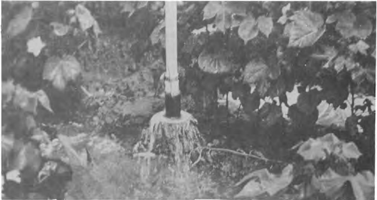
Figure 3. Nozzles attached to the end of the drop tubes typically operate at 1 to 5 psi and are designed to resist plugging.
