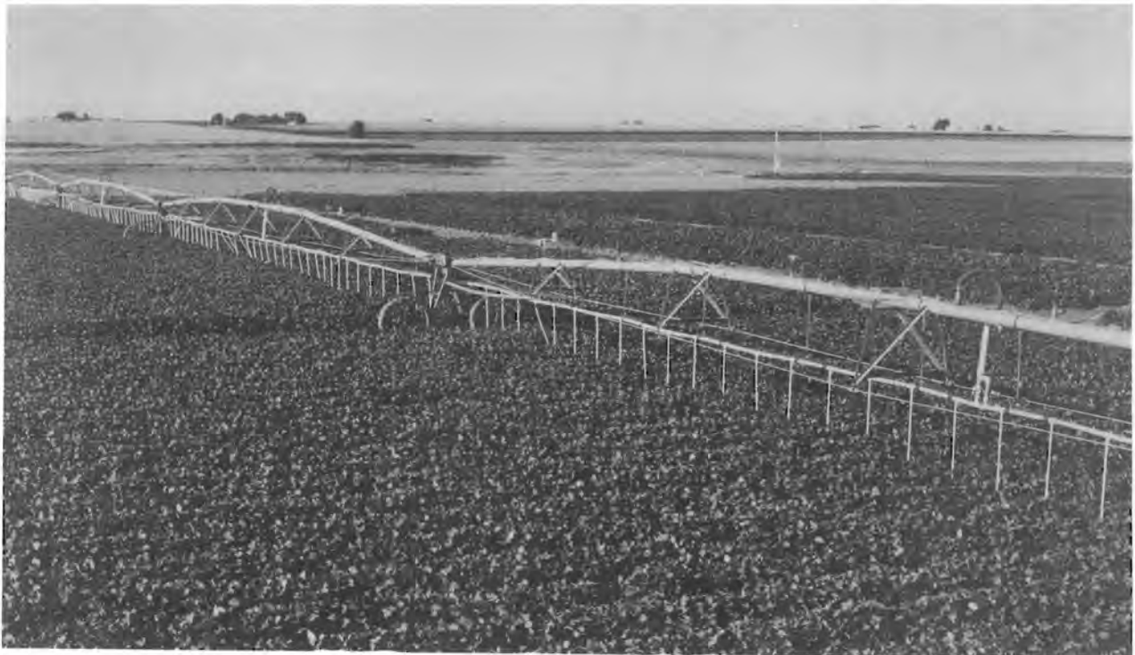
Figure 1. The low-energy, precision application (LEPA) irrigation system distributes water with great precision and economy through drop tubes suspended above the crop.
