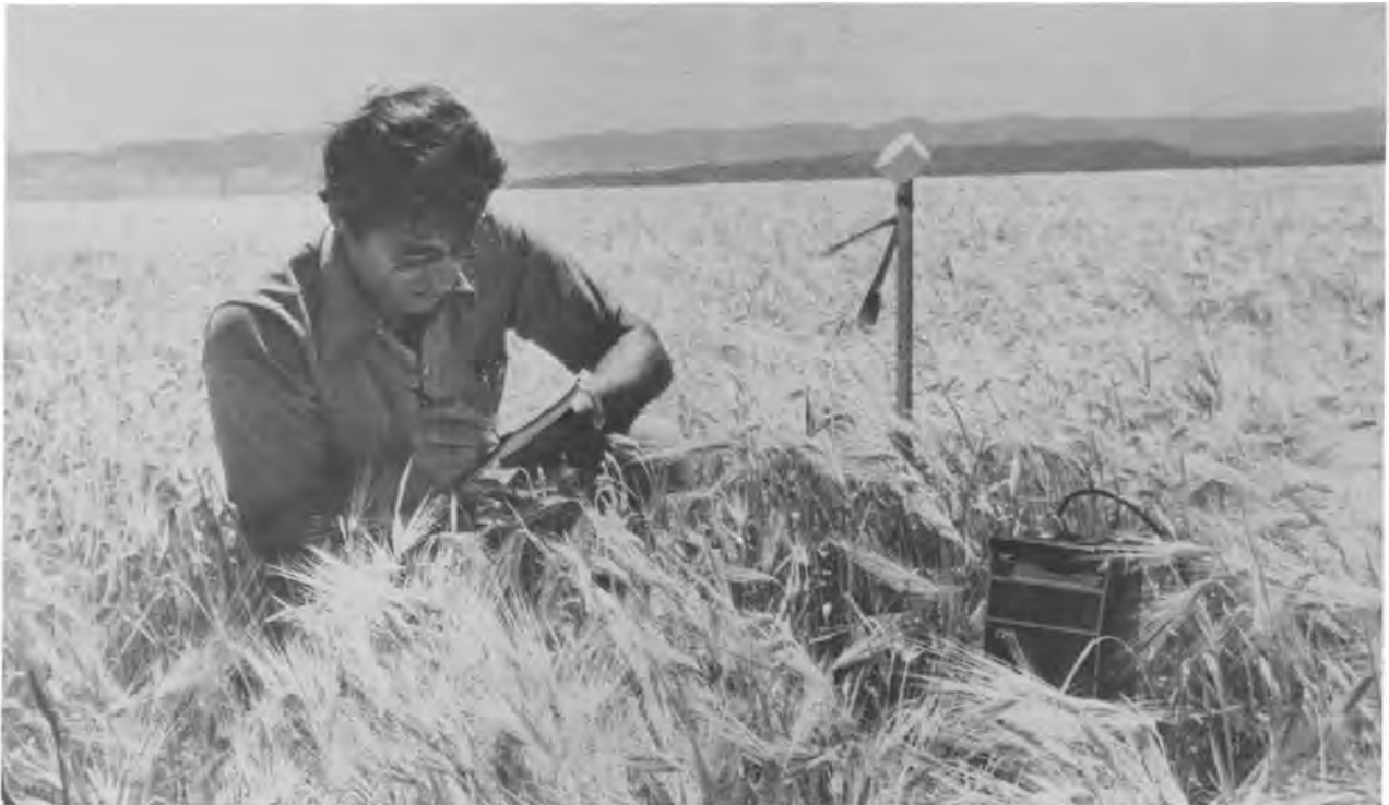
Figure 8. Using field data collected by this farmer, a computer will calculate an irrigation schedule and water application rate that produces ideal watering conditions for crop growth.
