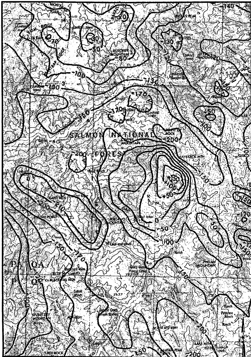
FIGURE 21. Aeromagnetic map of the study area (modified from U.S.G.S., 1975). Map is drawn with a 6.17 gamma/mile north and a 3.92 gamma/mile east regional trend removed. Magnetic contours are overlain on topography from the Elk City AMS map (scale 1:250,000). From Bennett, 1977, p.28.
