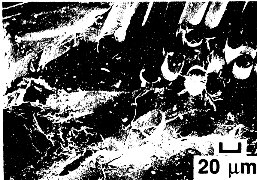
Figure 7. Matrix cracking in SiC-SiC material.
