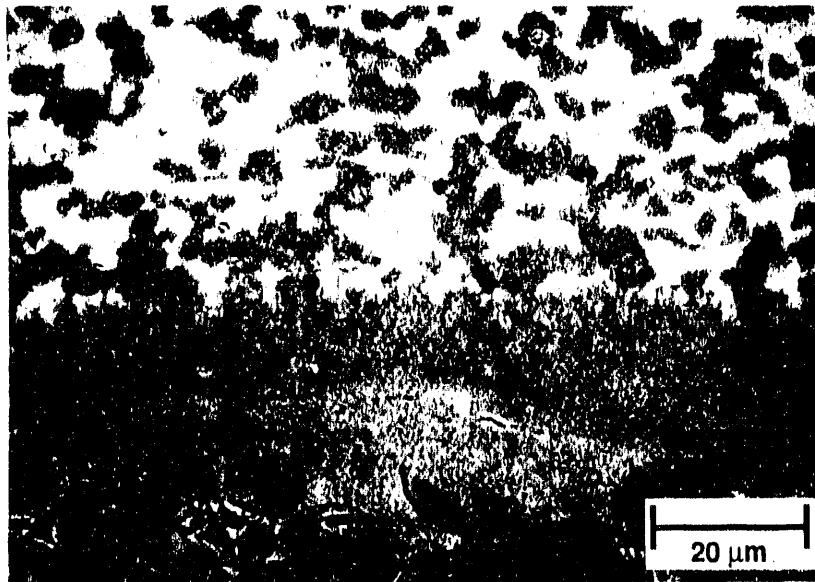
Figure 5. Higher magnification view of the interface between the SiC/SiC composite and the SiC+Si joint material produced by infiltrating a SiC+C powder mixture with Si.
