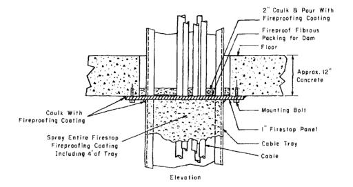
Fig. 14. Floor Penetration -
