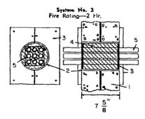
System number 3 is shown in Figure 5. The wall (1), forming materials (3) and fill, void, or cavity materials (4) are as described for system 1. The steel framing (2) is a mominal 6 inch directer, 0.25 inch wall steel pipe rigidly attached to the wall. The cables (5) are an aluminum conductor, PVC jacket 4/C, No. 14 AWG. There is a maximum 40 percent cable fill.
