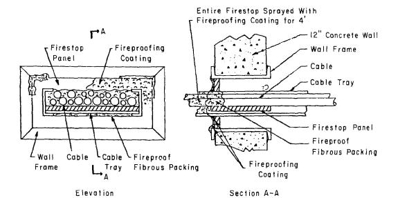
Fig. 12. Penetration Seal for Typical Prefabricated Channel Frame Wall Opening.
