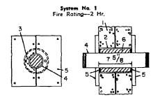
System number 1 is shown in Figure 3. The elements of this system are as follows: The wall (1) is nominally an 8 inch thick wall fabricated of concrete block, or common brick laid up with mortar. It must be a minimum 2
