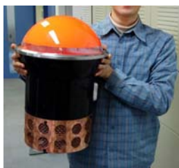
Fig. 5.1 Developing a small drifting buoy system with sea surface CO 2 sensors
