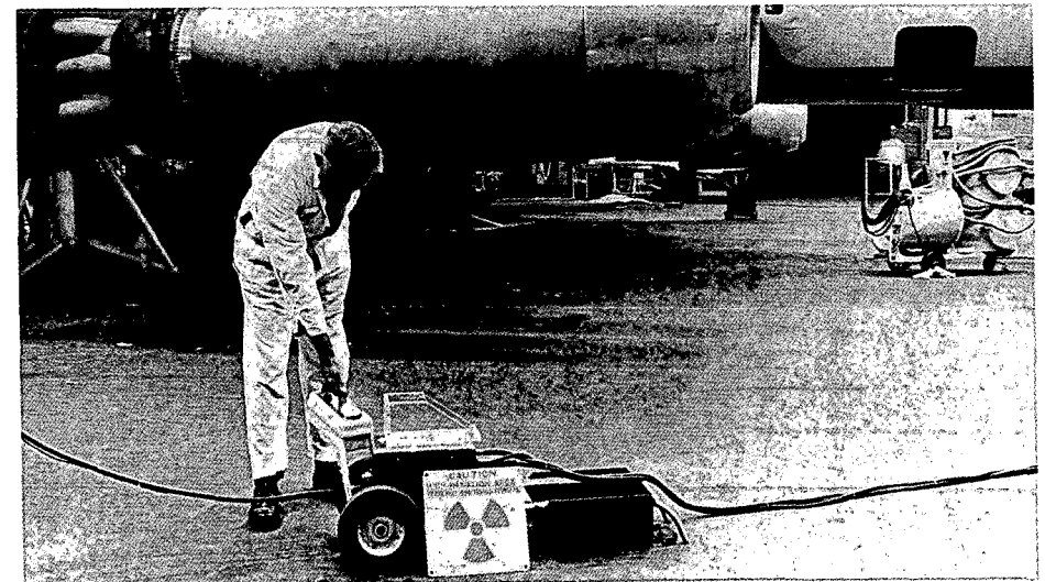
Figure 10. There are a number of reasons why a radiography source may be left exposed, but an exposed source does not necessarily have to result in an overexposure to radiation. Radiation surveys are performed to ensure that radiation levels are
