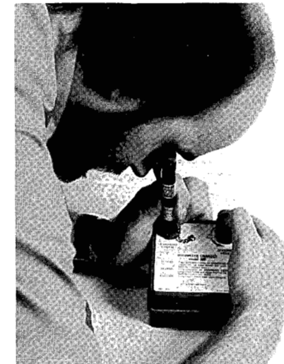
a) At the start of work, the radiographer charges his dosimeter. He will write down the dose that the dosimeter indicates.
