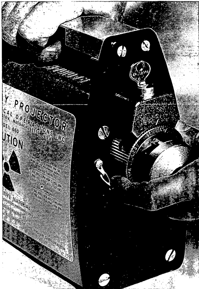
Figure 3. You cannot rotate the locking ring on this camera to lock it if the source is not in the fully shielded position.
