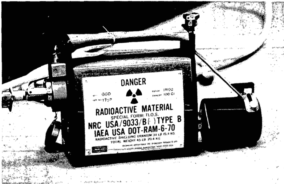
Figure 12. If the collimator can be attached directly to the camera (as in this picture), the source will always be at least partially shielded. The source will not travel through an unshielded guide tube.
