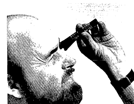
b) This radiographer is checking the reading on this pocket dosimeter. This is a good check from time to time to make sure you have not gotten excessive radiation exposure.
