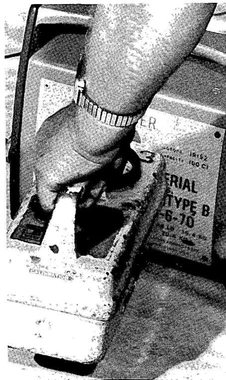
Figure 14. When a radiography source is received, a survey of surface radiation levels and radiation levels at 3 feet must be made. Here the radiographer makes sure his meter reads less than 200 mR/hr on all surfaces. The front of the camera where the source comes out is most important. If the source is not properly shielded, high radiation levels would be found at the front of the camera.
