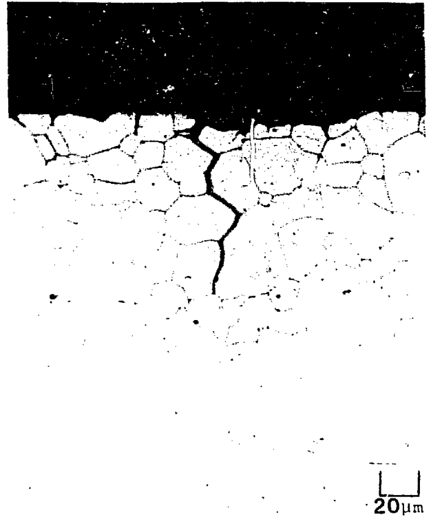
Fig. 3. Micrographs comparing the phenomena of (a) IGA and (b) SCC produced on MA C-rings in 10% NaOH + 0.1% Na 2 CO 3 solution at 300°C.
