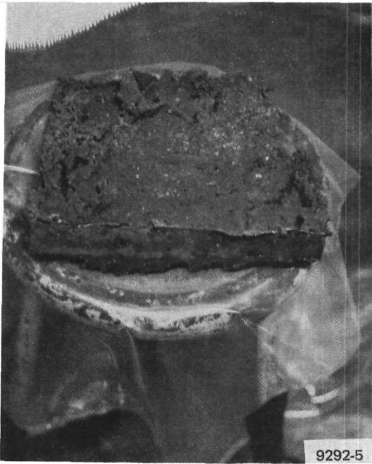
Figure 5. Stainless Steel Plate Covered with UO_2 (A thin copper sheet covered the plate previous to the pour.)
