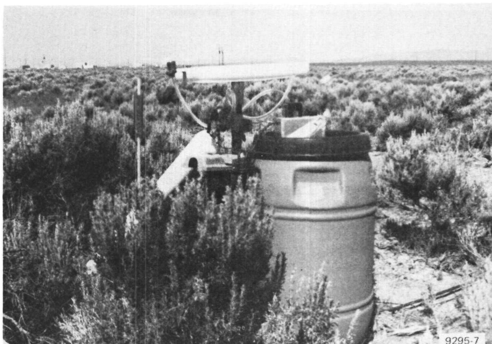
Figure 11. Typical Particle Sampling Station Positioned on Meteorological Grid
