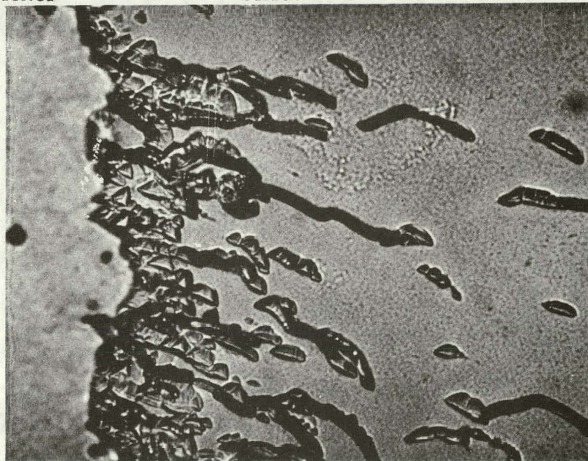
Wafer #83 (111) Tapered (10X) After Etch Nickel Silicon Wafer 1000 X
