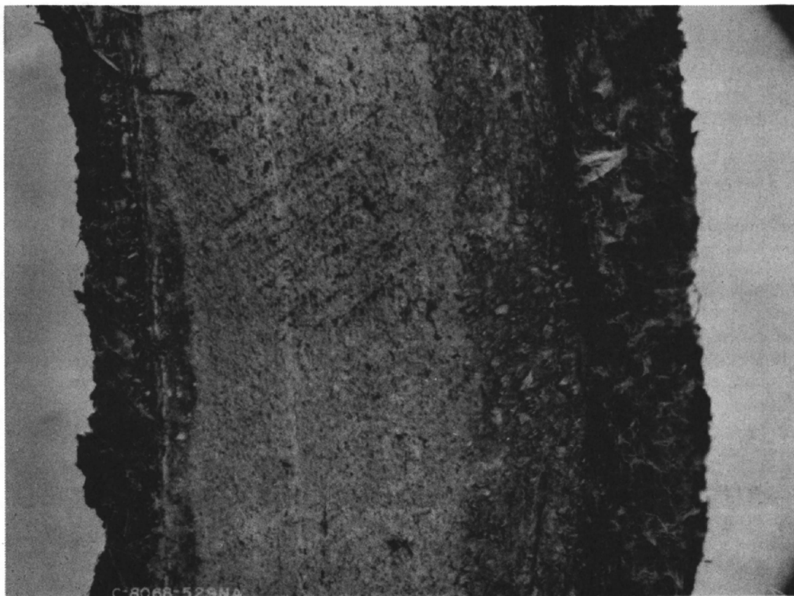
Figure VII-9. Photograph of asbestos-cement pipe showing alteration of outer surfaces (left and right sides). Photo PX-D-60860
