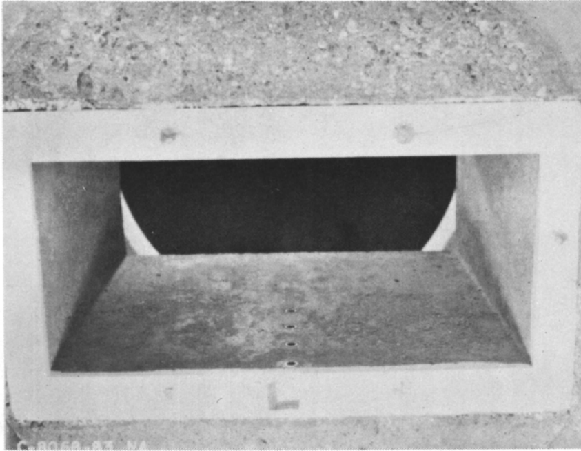
Figure III-63. Concrete orifice 4 by 9 by 8 inches prior to subjected continuous 10-feet-per-second flow of 100° F synthetic sea water. Photo PX-D-55286 NA
