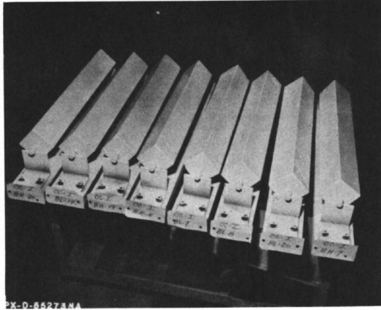
Figure V-3. Concrete test bars coated with silicone alkyd coating, Material No. IV, are shown before exposure. Photo PX-D-55273 NA
