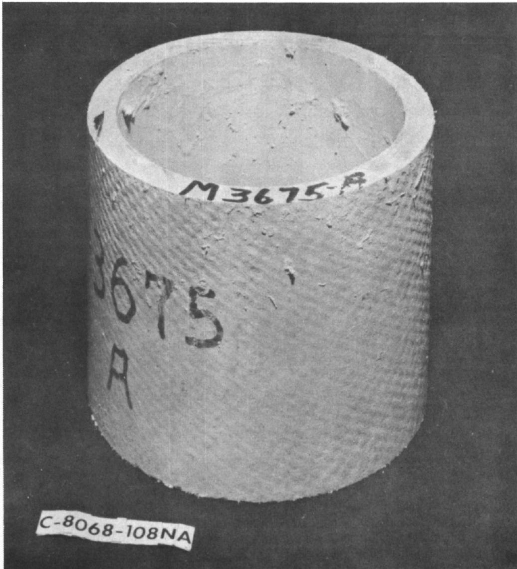
Figure III-69. Typical 8-inch-diameter section of asbestos-cement pipe as tested in the 290° F brine. Photo PX-D-55291 NA
