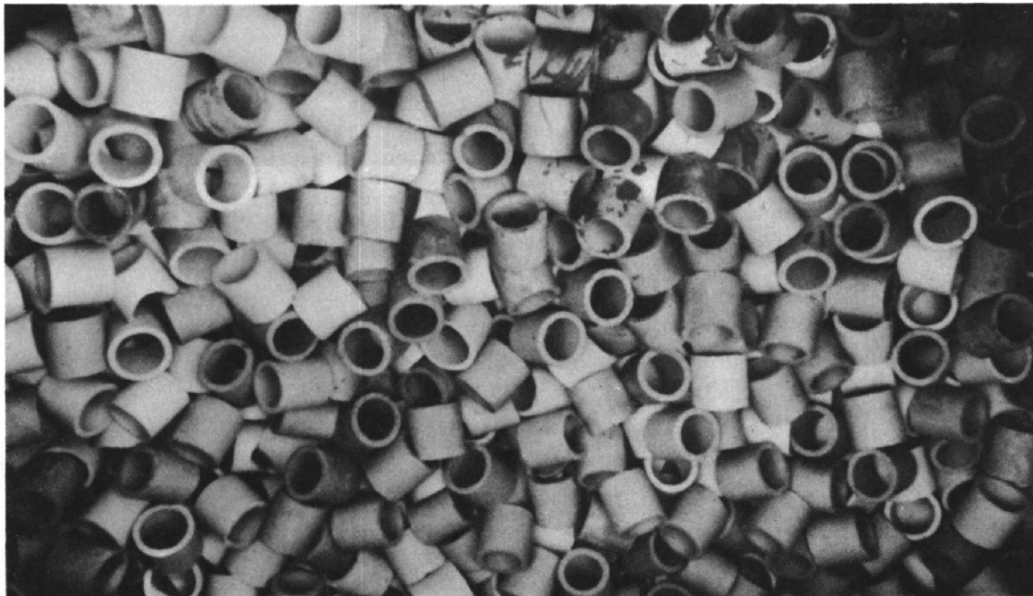
FIGURE 3-13. DEAERATOR TOWER PACKING
