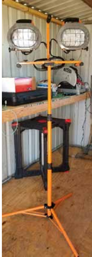
Figure 3.5 : 1000W twin-head halogen yellow work light
