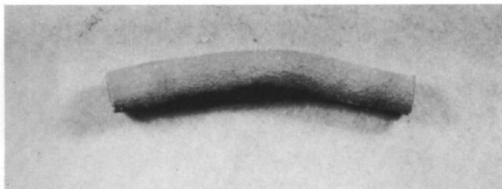
Specimen AH-1-4, Swaged, Furnace Cooled, and Gamma Quenched, after 0.046 a/o Burnup at 130°C
