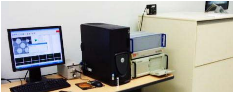
Fig. 1.1. A Nanoindentation apparatus for nano-scale mechanical measurements (MTS Nano indenter XP®).
