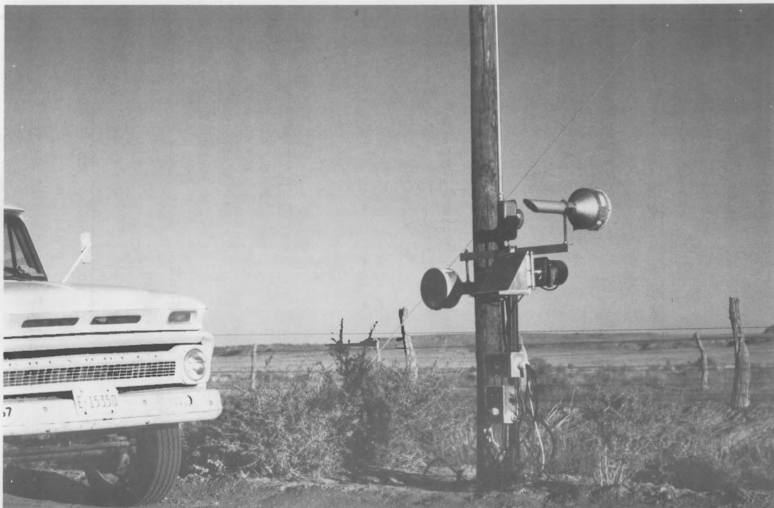
FIGURE 13. A North Fence Sampling Site with View Towards Northwest Showing Isokinetic Sampler and South- and North-Facing Air Impact Flow Particle Collectors
