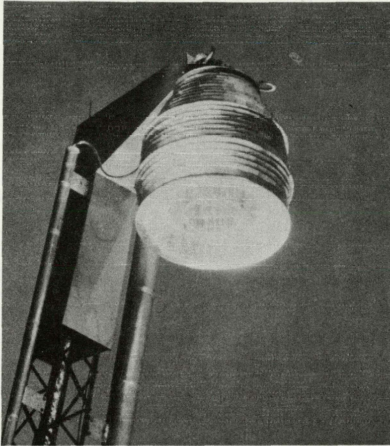
Figure 17. Photograph of Boiler-Superheater of the DOE Advanced Components Test Facility at Georgia Tech - Designed by Professor Francia.
