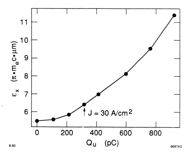
Fig. 5. Emittance versus charge per bunch.
