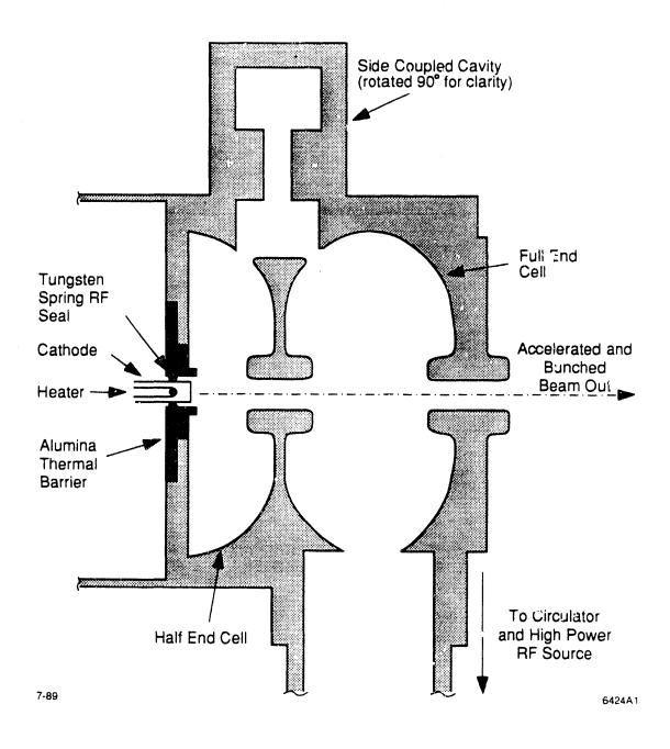
Fig. 1. Cross section of the gun cavity.
