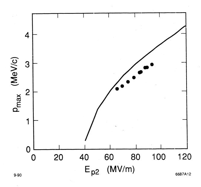
Fig. 8. Maximum momentum versus peak electric field.
