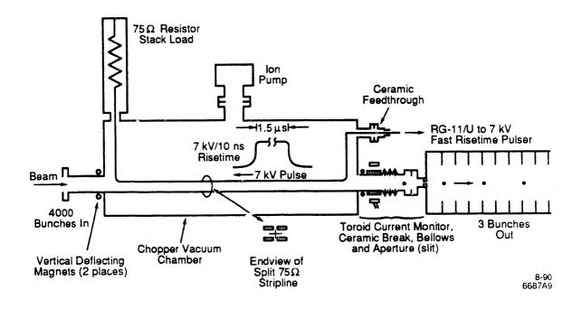
Fig. 4. Side view of the chopper.
