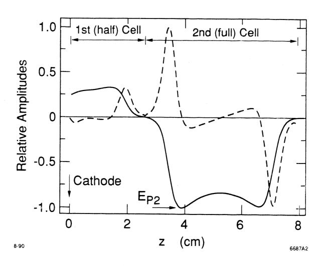
Fig. 2. Radial (dashed) and longitudinal (solid) electric field profiles for the RF gun.
