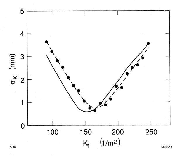
Fig. 6. Measured (points) and simulated (line) horizontal beam size,  $\sigma_x$ , versus quadrupole (GTLQ4) strength parameter,  $K_1$  for beam parameters: p = 2.7 MeV/c,  $\Delta p/p = \pm 10\%$  and  $\hat{I} = 100 \text{ mA}$ . The normalized rms emittances then are 39 mm·mrad (measured) and 26 mm·mrad (simulated).
