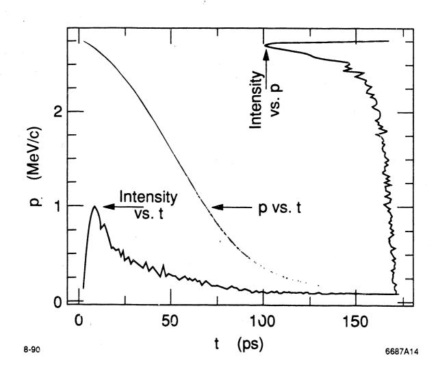
Fig. 7. Gun longitudinal phase-space.
