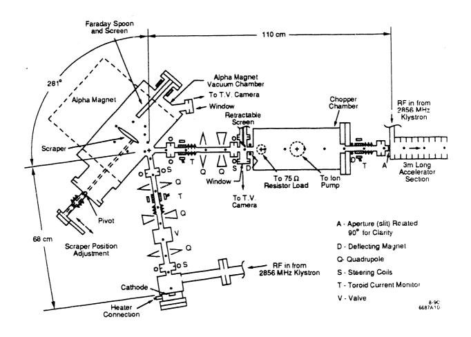
Fig. 3. Gun-to-linac layout.
