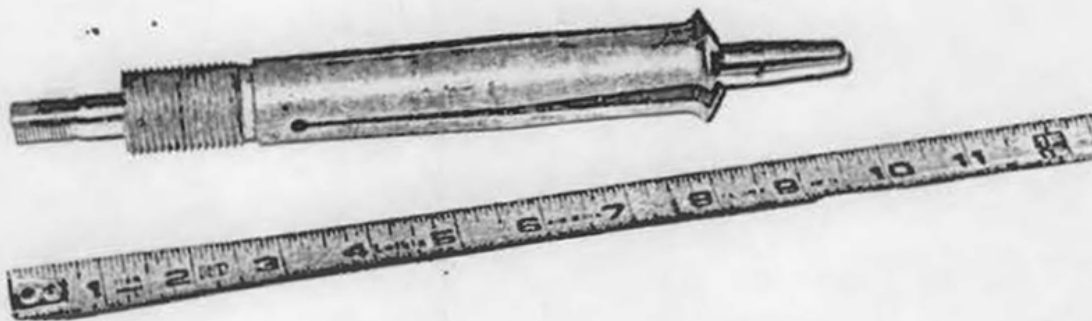
FIGURE 5. Push Rod Inserted into Bit To Expand Spalling Wedge
