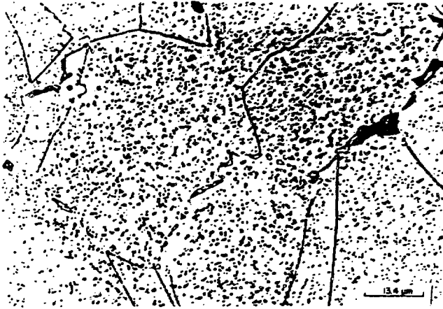
Fig. 10. Optical micrograph showing large amounts of carbide precipitation within the matrix and large sigma phase particles at the grain boundaries in the stressed region of type 304 stainless steel during 7.3 \times 10^4 h (about 8 1/2 years) at 593°C (1100°F) and 117 MPa.
