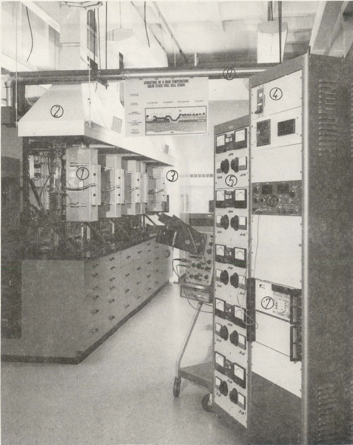
Fig. 5.22 General View of 5-Station HTSOE Fuel Cell Life Test Facility (Left) and Control and Data Acquisition System (Right)
