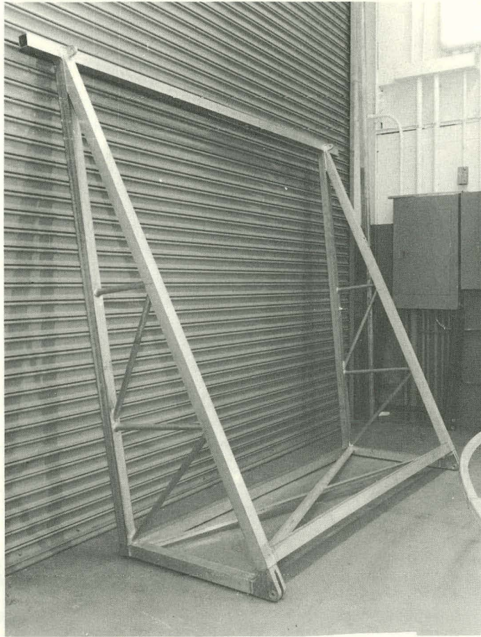
Figure 31. Wedge pivot structure of heliostat assembly.
