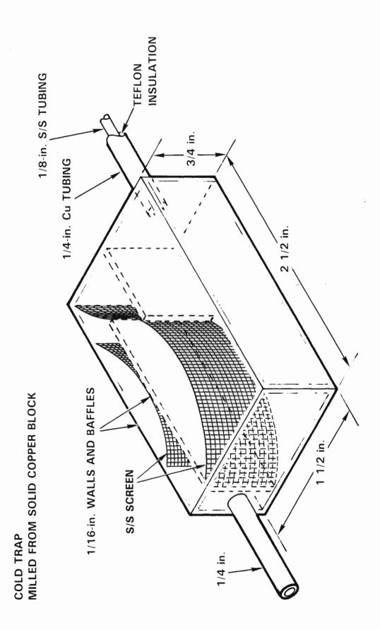
FIGURE 1. Final cold trap design
