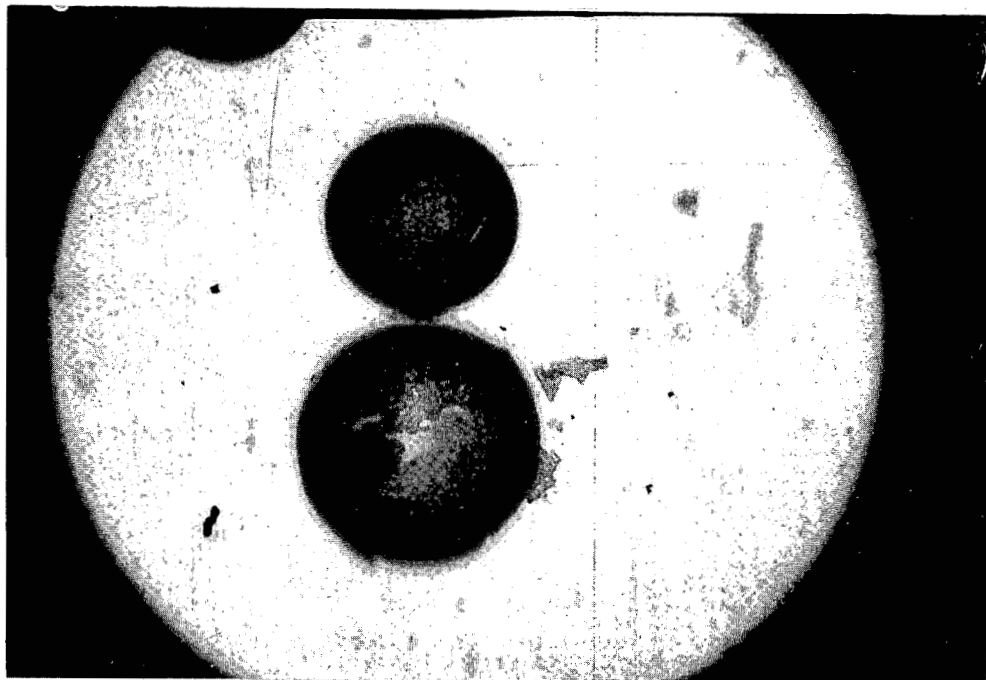
Fig. 4.9 Silicone-Coated Beads after CaCO 3 Scale has Covered Them (magnification: x 50)
