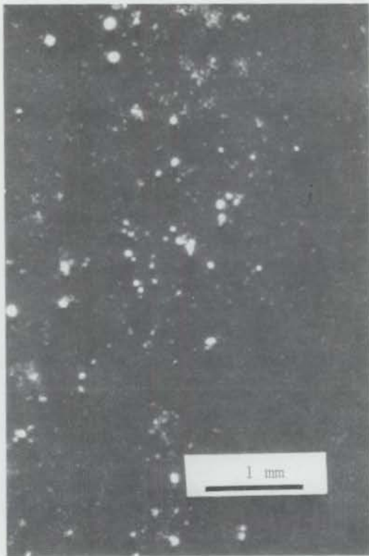
FIGURE 1. Photomicrograph of Track-Etch Film to Which a Plutonium Concentration Grade of "2" was Assigned.
