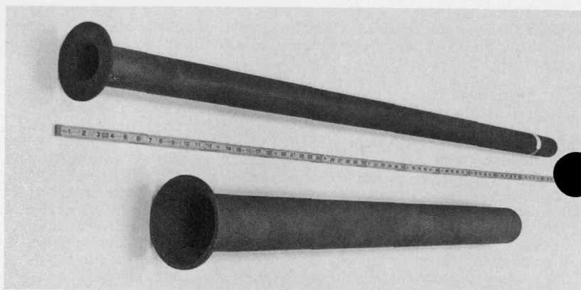
Figure 7. Comparison of the Inner (Top) and Outer (Bottom) Tubes Used in the Prototype Tests
