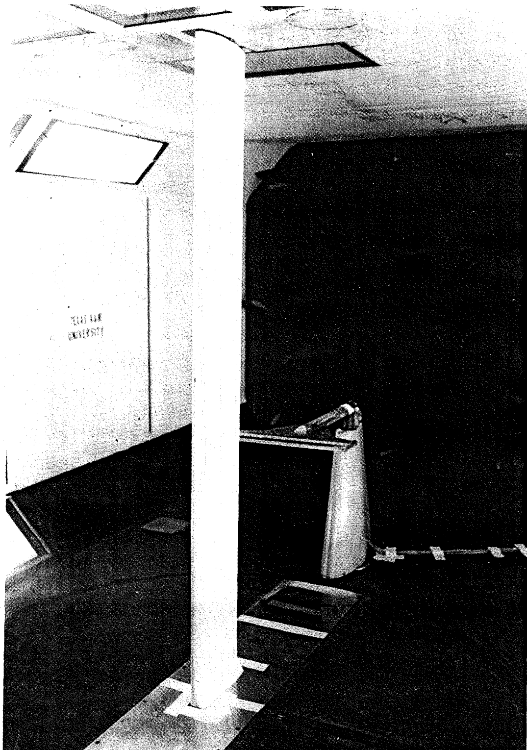
Figure 2-2. Blade Model Mounted in the Wind Tunnel Test Section
