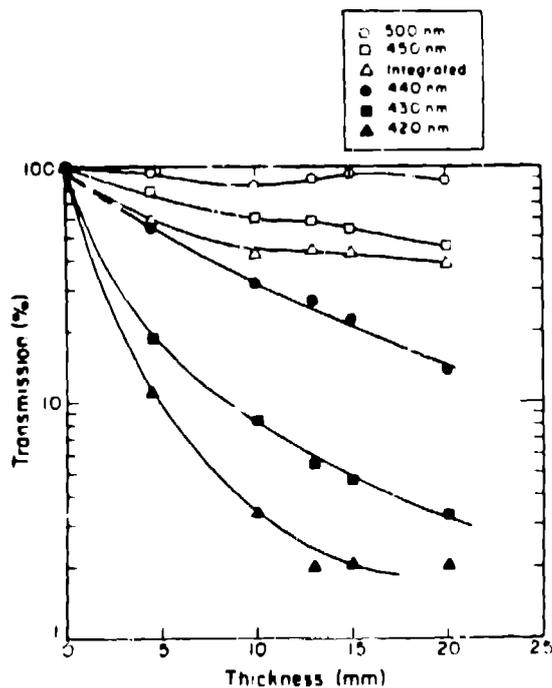
Fig. 4. Optical transmission at various wavelengths for differing thicknesses of BBQ in acrylic.
