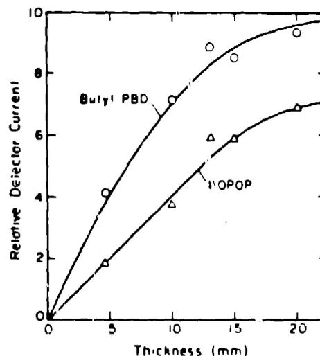
Fig. 5. Relative light collected at end of BBQ acrylic of various thicknesses, for two different incident light spectra from liquid scintillators. In both cases, the  $^{60}\text{Co}$  gamma irradiation was held constant.
