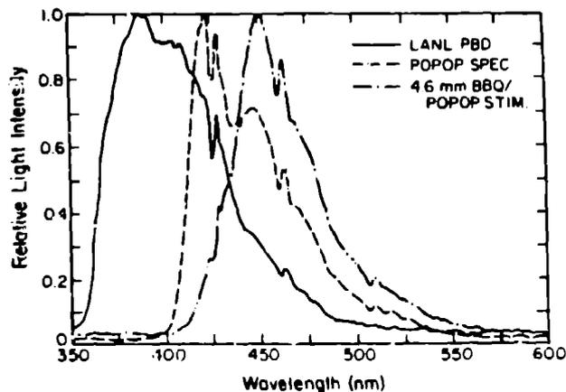
Fig. 3. Normalized emission spectra of two liquid scintillators, produced by  $^{60}\text{Co}$  gamma radiation, in comparison with stimulated emission from BBQ acrylic.
