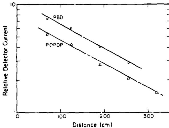
Fig. 6. Observed dependence of detector current on BBQ acrylic distance, when stimulated by differing spectra from liquid scintillators. The thickness of BBQ was 12.5 mm in a semicircular shape. The positions of the liquid scintillator light on the BBQ is illustrated in Fig. 2.
