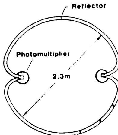
Fig. 2. Acrylic BBQ scintillator shape. Thickness is 12.5 mm. Positions of light source for current measurements are indicated by "X."
