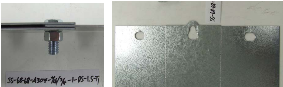
Figure 4.37 Failure mode of test SS-68-68-A307-9/16x3/4-1-DS-1.5-T1.
