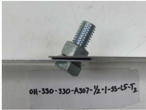
Figure 4.8 Sheet shear failure of single shear connection OH-330-330-A307-1/2-1-SS-1.5-T2.
