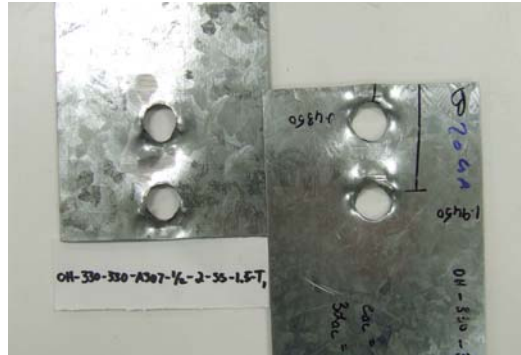
Figure 4.11 Failure mode of test OH-330-330-A307-1/2-2-SS-1.5-T1.
