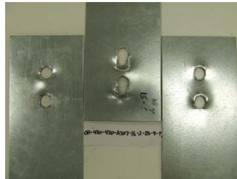
Figure 4.6 Sheet bearing failure of double shear connection OH-430-430-A307-1/2-2-DS-4-T1.
