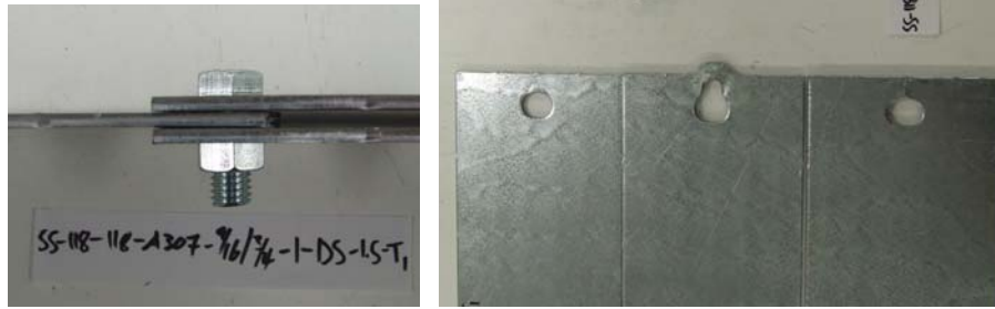
Figure 4.35 Failure mode of test SS-118-118-A307-9/16x3/4-1-DS-1.5-T1.
