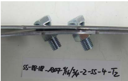
Figure 4.21 Failure mode of test SS-118-118-A307-9/16x3/4-2-SS-4-T2.
