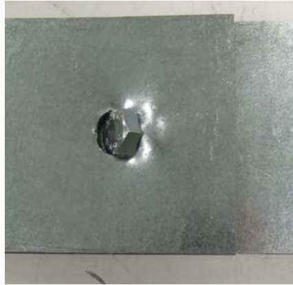
Figure 4.19 Failure mode of test SS-118-118-A307-9/16x3/4-1-SS-4-T2.
