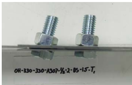
Figure 4.12 Failure mode of test OH-330-330-A307-1/2-2-DS-1.5-T1.
