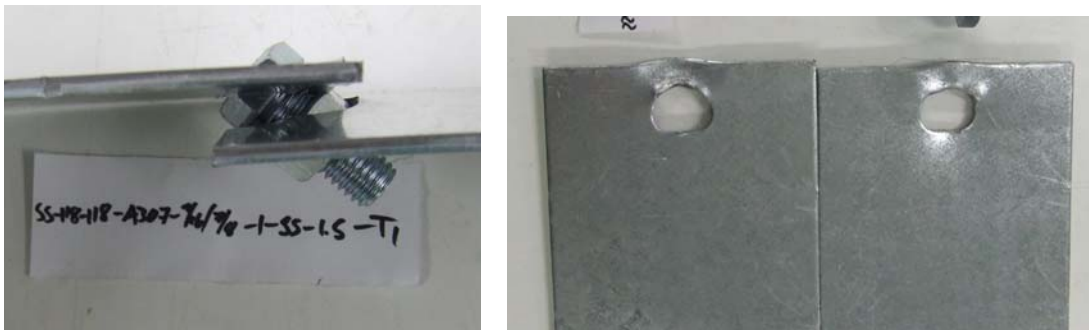
Figure 4.32 Failure mode of test SS-118-118-A307-9/16x7/8-1-SS-1.5-T1.
