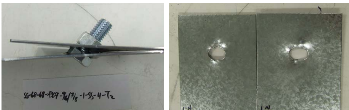
Figure 4.18 Failure mode of test SS-68-68-A307-9/16x7/8-1-SS-4-T2.
