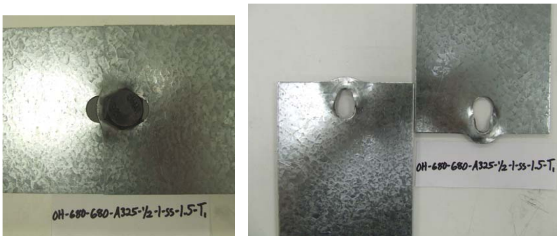
Figure 5.11 Sheet shear failure of a 68 mil single shear connection with one A325 bolt.
