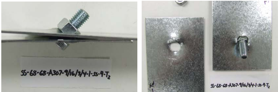
Figure 4.17 Failure mode of test SS-68-68-A307-9/16x3/4-1-SS-4-T2.
