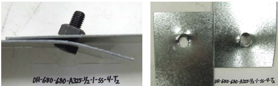
Figure 5.9 Bearing failure of a 68 mil single shear connection with one A325 bolt.
