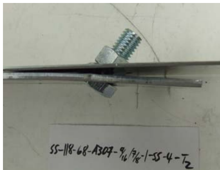
Figure 4.23 Failure mode of test SS-118-68-A307-9/16x7/8-1-SS-4-T2.
