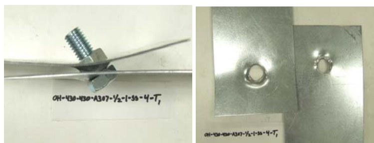
Figure 4.2 Sheet bearing failure of single shear connection OH-430-430-A307-1/2-1-SS-4-T1.
