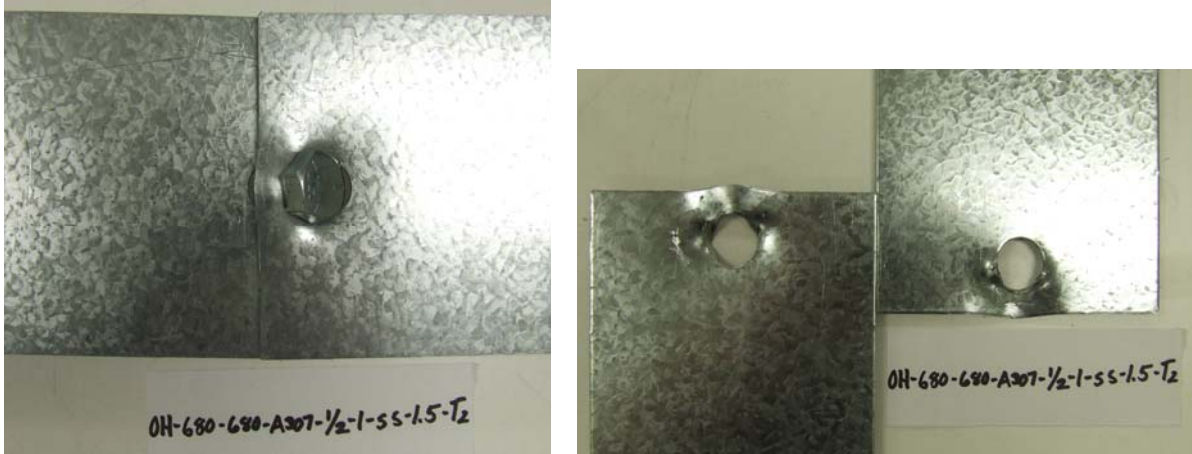
Figure 5.10 Sheet shear failure of a 68 mil single shear connection with one A307 bolt.
