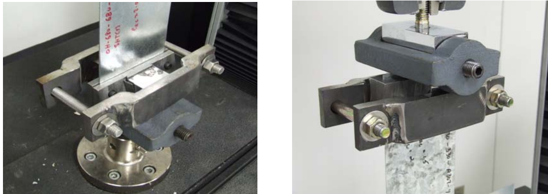
Figure 3.2 Bottom fixture and top fixture.
