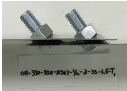
Figure 4.11 Failure mode of test OH-330-330-A307-1/2-2-SS-1.5-T1.
