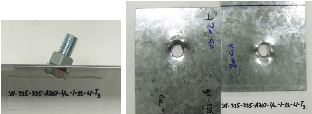
Figure 4.15 Failure mode of test SH-33S-33S-A307-1/2-1-SS-4-T3.
