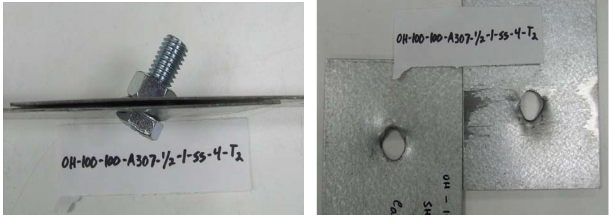
Figure 5.7- 39 mil low ductile steel bearing failure.
