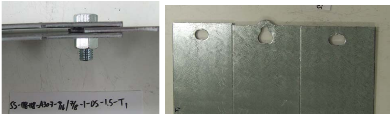
Figure 4.36 Failure mode of test SS-118-118-A307-9/16x7/8-1-DS-1.5-T1.
