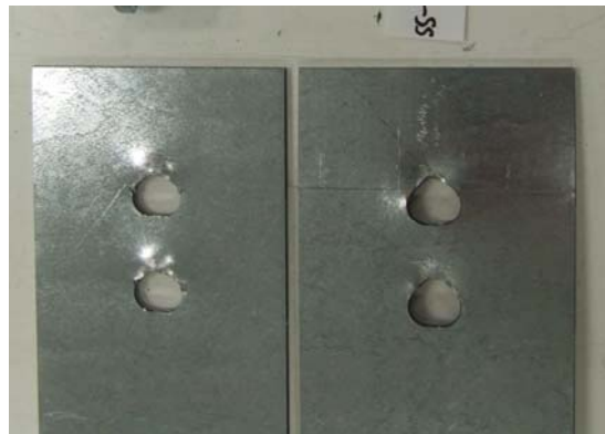
Figure 4.21 Failure mode of test SS-118-118-A307-9/16x3/4-2-SS-4-T2.
