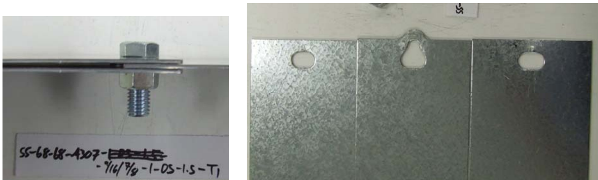
Figure 4.38 Failure mode of test SS-68-68-A307-9/16x7/8-1-DS-1.5-T1.
