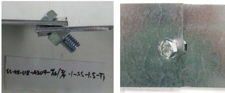
Figure 4.31 Failure mode of test SS-118-118-A307-9/16x3/4-1-SS-1.5-T1.
