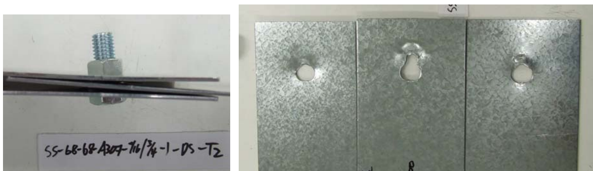
Figure 4.26 Failure mode of test SS-68-68-A307-9/16x3/4-1-DS-4-T2.
