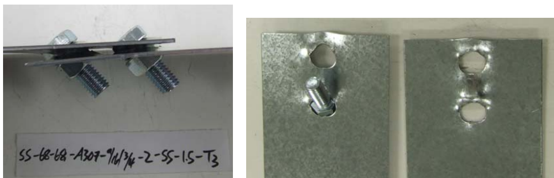
Figure 4.39 Failure mode of test SS-68-68-A307-9/16x3/4-2-SS-1.5-T3.
