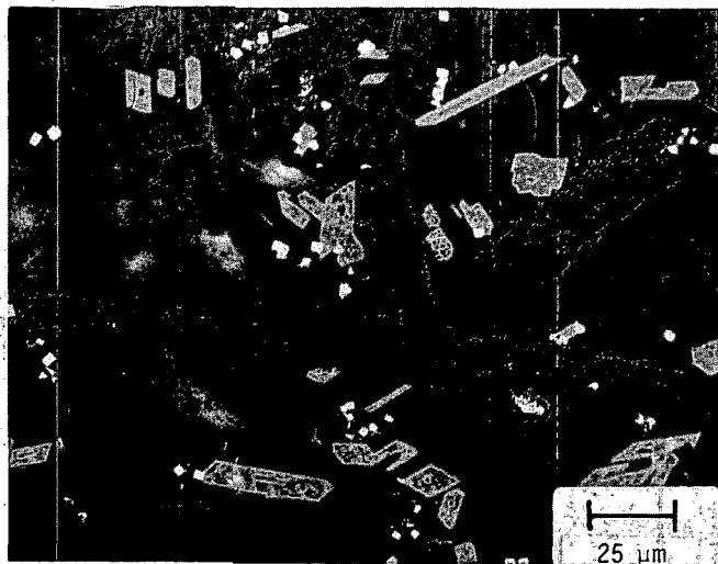
FIGURE 12. Microstructure of 77-260 Waste Glass Doped with 2 wt% ^{244}Cm and Slow-Cooled at -6.25^\circ C/hr (a)
