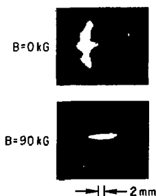
Fig. 2. Carbon fiber target coated with a thin layer of aluminum for which the highest gain was observed. Framing images of the \text{CO}_2 laser-fiber interaction at B = 0, 90 kG.
