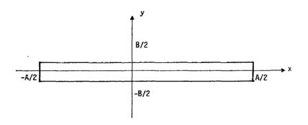
Length of the slit is taken along the x direction while the height is taken along the y direction.
