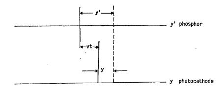
The coordinate transformation between the photocathode and phosphor is given below
