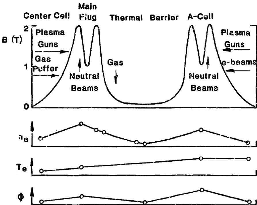
Fig. 5 TMX thermal barrier related experiment, with schematic illustration of possible diagnostic measurements.
