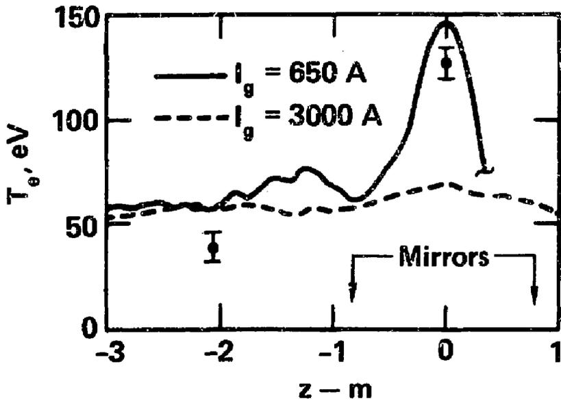
Fig. 3 Electron temperature axial profiles for typical 2XIB gas box current. The curves are Monte Carlo calculations.
