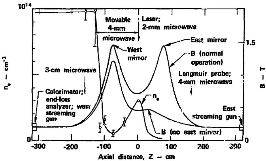
Fig. 4 Axial density profiles measured in 2X11B.
