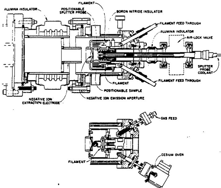
Fig. 19. Schematic drawing of the ORNL University of Aarhus geometry cesium-plasma negative ion sputter source [Ref. 57].
