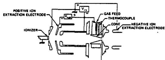
Fig. 17. Schematic drawing of the Middleton-Adams negative sputter ion source [68].
