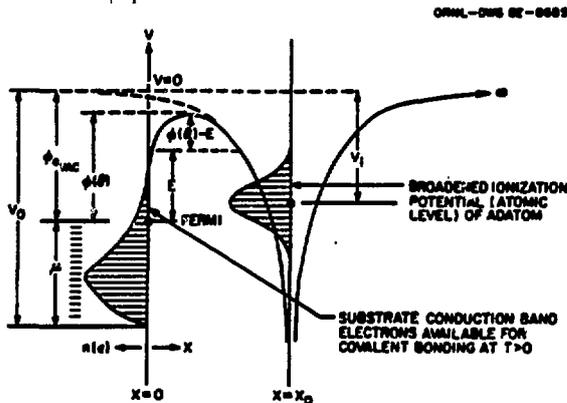
Fig. 14. Simplified potential energy diagram of a sputtered atom interacting with an electropositive adsorbate covered surface (tunneling theory).
