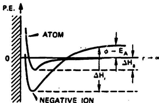
Fig. 11. Potential energy curves for an electronegative atom and ion as a function of distance from a hot metal surface.
