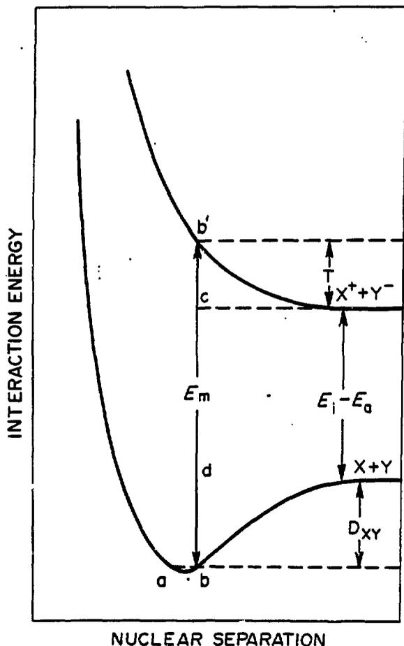
Fig. 1. Potential energy curves for a molecule and ion fragments illustrating the polar dissociative electron attachment process.
