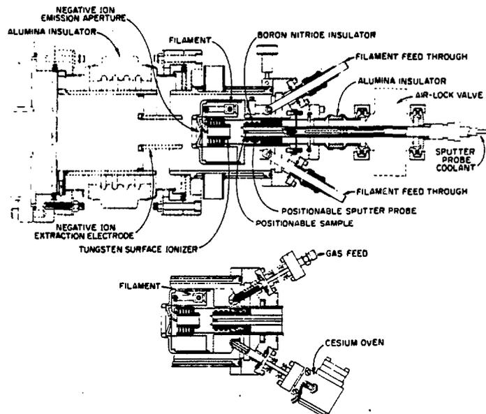
Fig. 20. Schematic drawing of the ORNL axial geometry cesium-plasma negative ion sputter source [Ref. 91].
