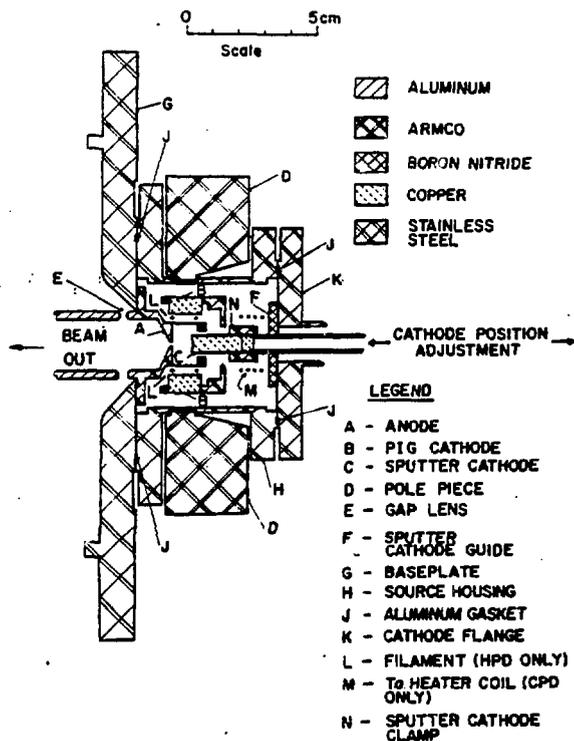
Fig. 21. Schematic drawing of the cold cathode University of Aarhus geometry negative ion sputter source of Smith [Ref. 93].
