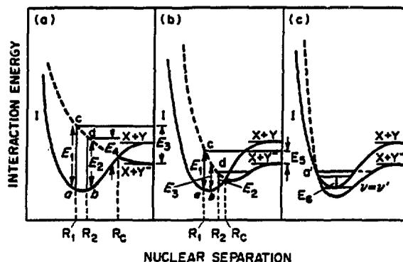
Fig. 2. Potential energy curves illustrating three ways for electron dissociative attachment of a molecule.
