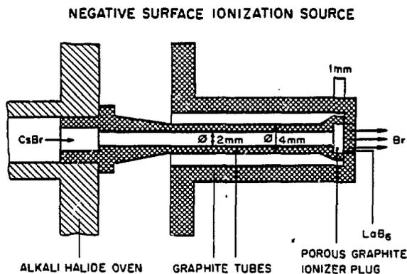
Fig. 12. Schematic diagram of thermodynamic equilibrium type negative ion source [64].
