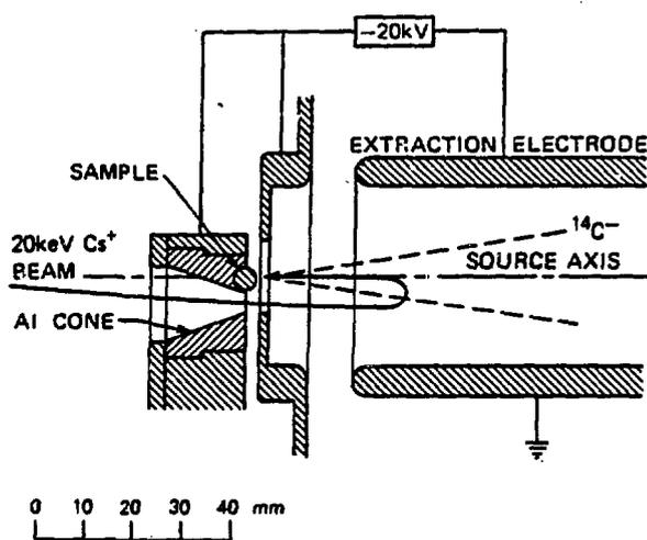
Fig. 18. Schematic drawing of the refocus-geometry Middleton-Adams source [Ref. 87] operated in the reflected beam mode.
