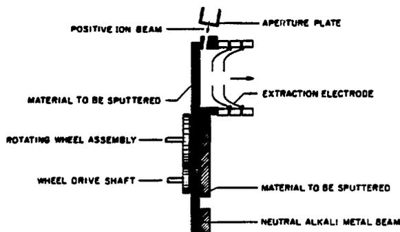
Fig. 16. Schematic drawing of the Mueller-Hortig negative sputter ion source [84].
