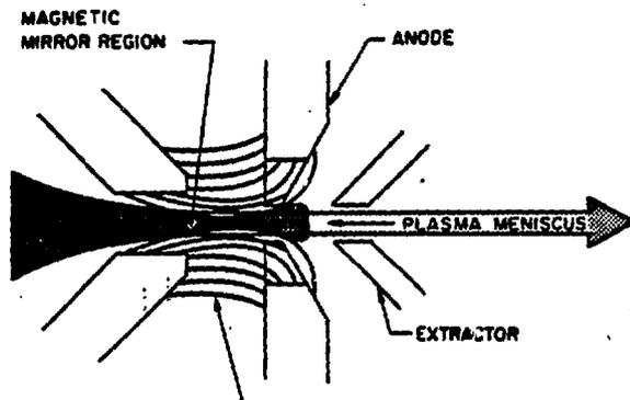
Fig. 3. Schematic drawing of the plasma and ion extraction region of the duoplasmatron ion source.
