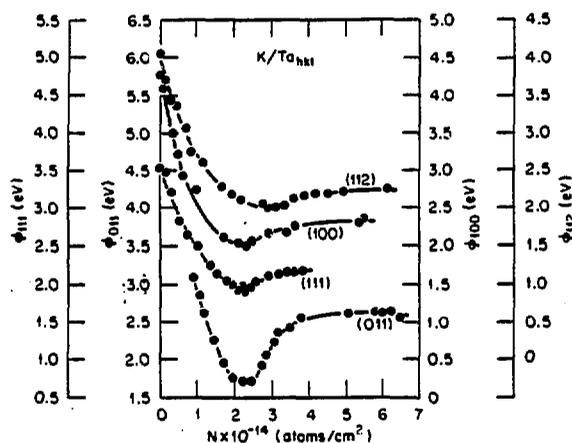
Fig. 10. Illustration of the effect of electropositive atom adsorption on the work function  $\phi$  of single crystal Ta as a function of fractional surface coverage,  $\theta_c$  [Ref. 54].
