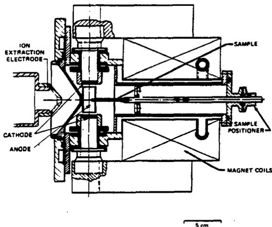
Fig. 4. Schematic drawing of a direct-extraction radial-Penning-discharge negative ion source [Ref. 33].
