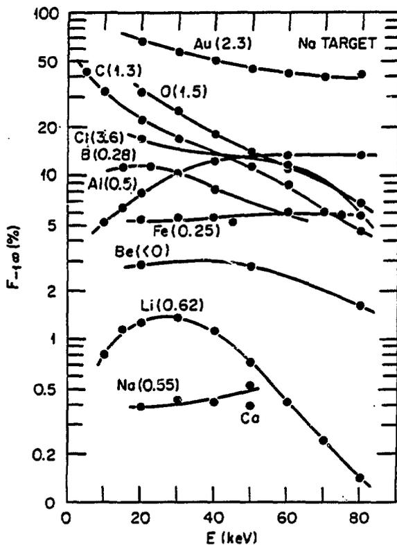
Fig. 6. Negative ion equilibrium charge exchange fractions versus ion energy for several ions in sodium exchange vapor [Ref. 43].
