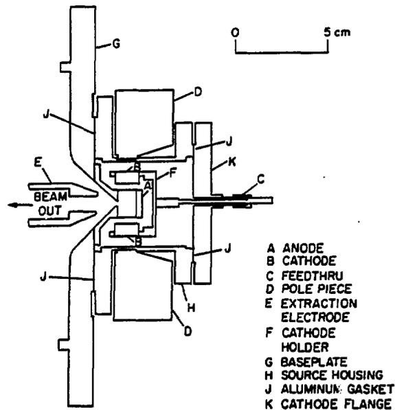
Fig. 5. Schematic drawing of a direct-extraction radial-Penning-discharge negative ion source [Ref. 34].
