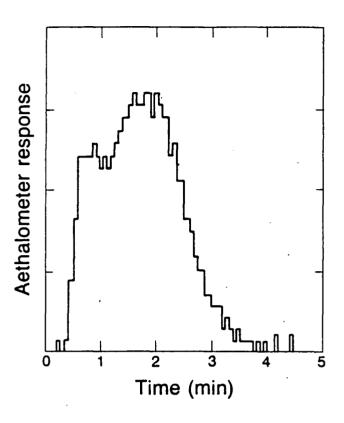
Fig. 2. Aethalometer response during transit of a plume from agricultural burning over the Bahamas. The aethalometer time-base period of 4 seconds gives a horizontal resolution of approximately 500 m.
