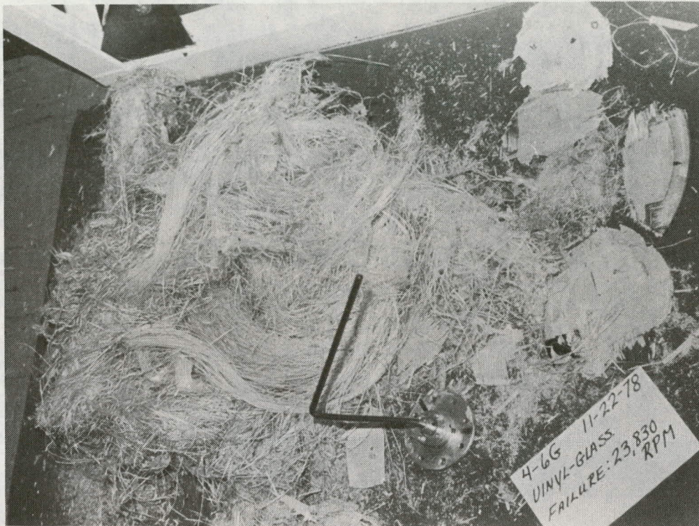
Fig. 25 Typical failure mode of vinyl-glass flywheel.
