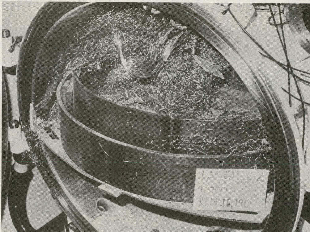
Fig. 30 Typical failure mode of steel-wire flywheel.
