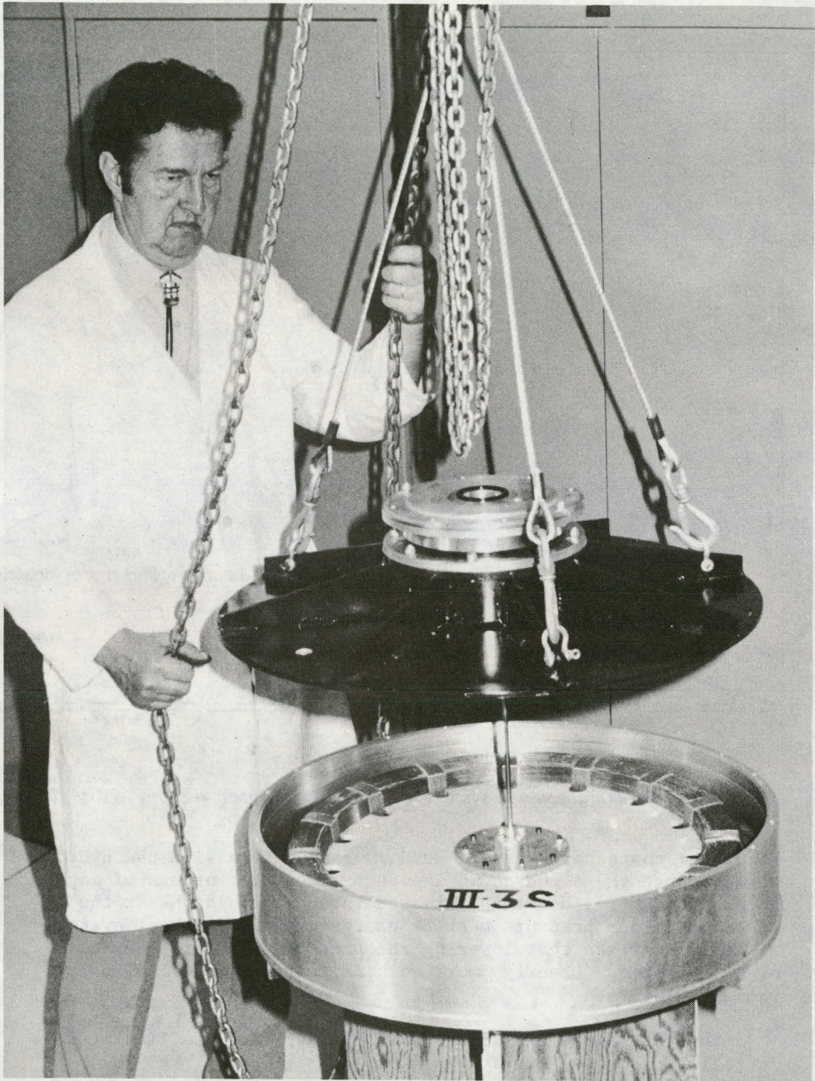
Fig. 49 Energy-storage system 2 with final flywheel.
