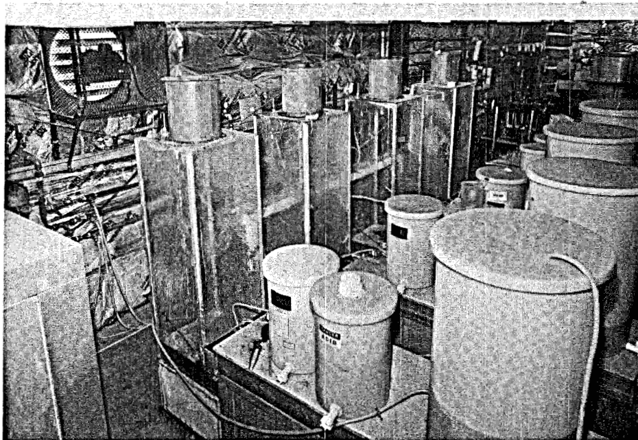
FIGURE 4 WATER CHEMISTRY LABORATORY Pilot Cooling Towers used for Establishing Water Treatment and Corrosion Tests (tubes in heat exchangers on the wall)
