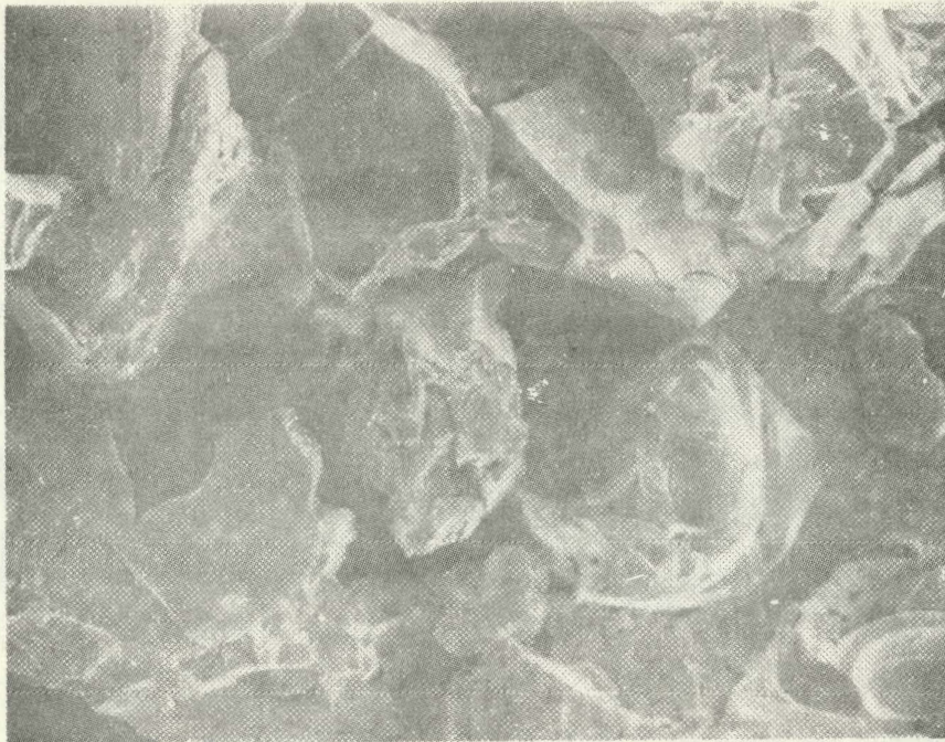
Figure 10.-- \text{LaCrO}_3 Prepared from Polyhydroxy-Resin Precursor with Ethylene Glycol Present, Heated at 923 K for 4 Hours; (100X magnification)
