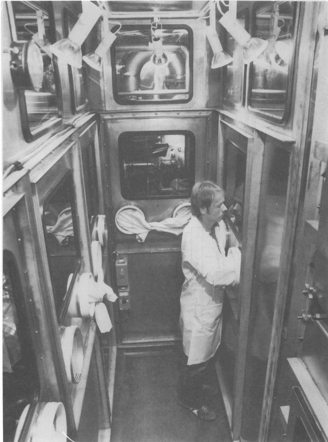
FIGURE 17. Removable Containment Module for the PSRT Off-Gas Treatment System
