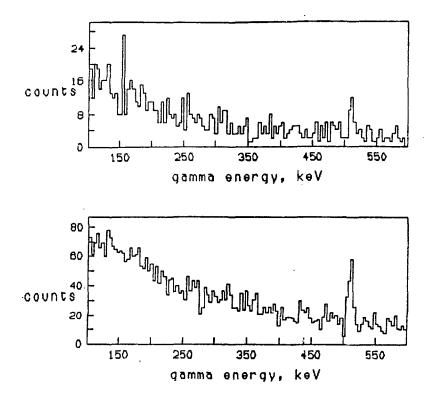
Fig. 7. The Yray spectrum Λ<sup>10</sup>Β from in the (a) bound state region, -12<BA<+6 MeV and **(b)** from the region 6<BA<24 MeV. The (K, m) coincidence window is 80 ns wide.
