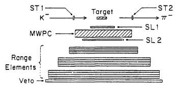
Fig. 11. Experimental apparatus for the lifetime measurement on  $^{12}C$ .
