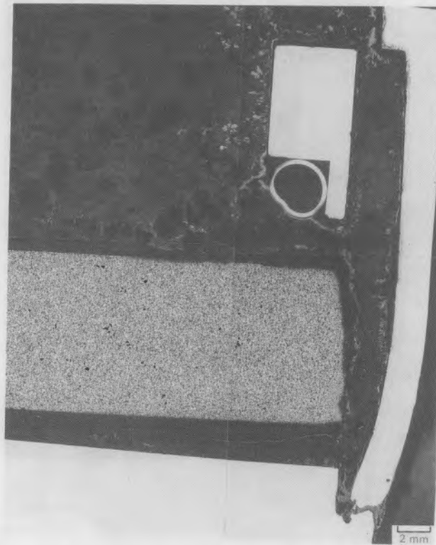
FIGURE 5. Macrographic Cross Section of Inner Capsule in Vicinity of Failed Weld
