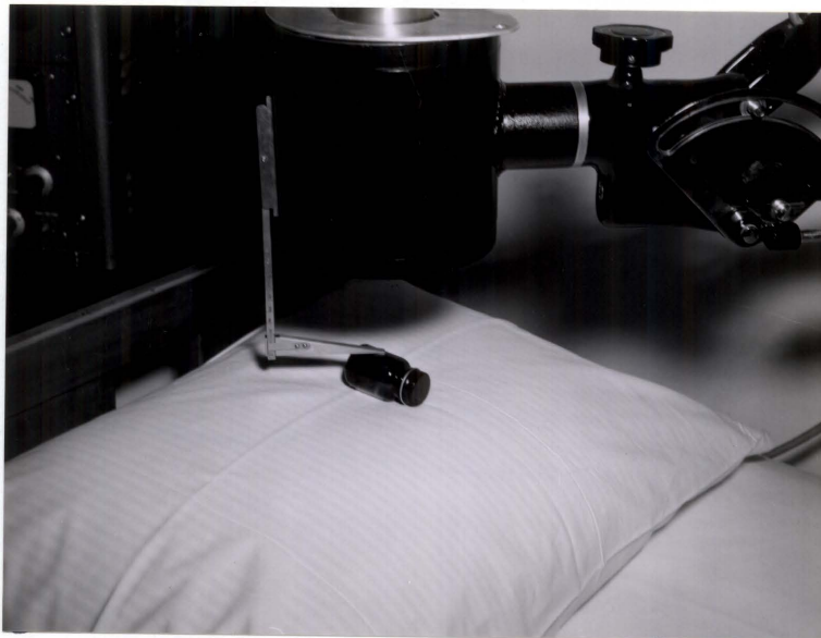
Fig. 5--Scintillation head and relative position of standard employed in thyroid uptake studies.
