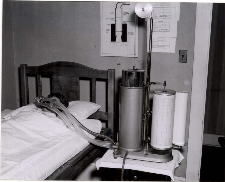
Fig. 1--Benedict-Roth type of spirometer employed in determination of basal metabolic rate.
