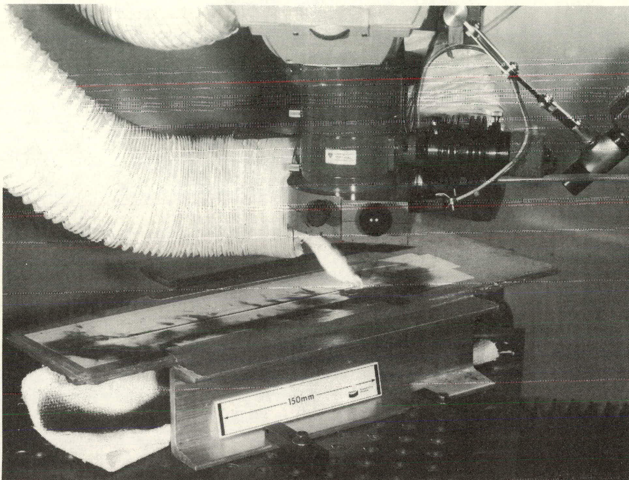
Figure 4. Laser Cutting Contour and Holes in 6.35-mm-Thick Kevlar/Epoxy Laminate (Cycle Time = 75.0 Seconds Per Part)
