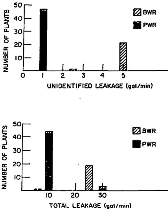
Figure 1. Amounts of Unidentified and Total Coolant Leakage Allowed at BWRs and PWRs. Conversion factor: 1 gal/min = 3800 cm<sup>3</sup>/min.
