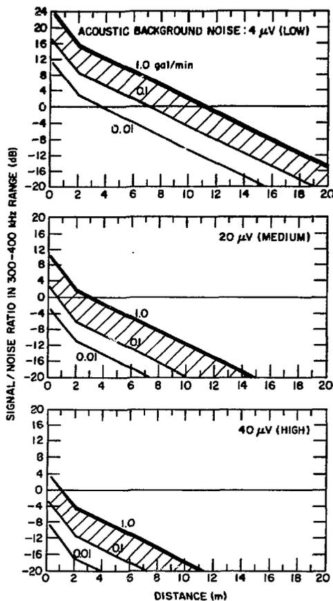
Figure 3. Predicted Acoustic Signal-to-Noise Ratios vs Distance along a 10-in. Schedule 80 Pipe for Three Leak Rates and Three Levels of Estimated Acoustic Background Noise. The striped areas indicate possible enhancement of the signal for the 0.1 gal/min leak because of the presence of reflective insulation.
