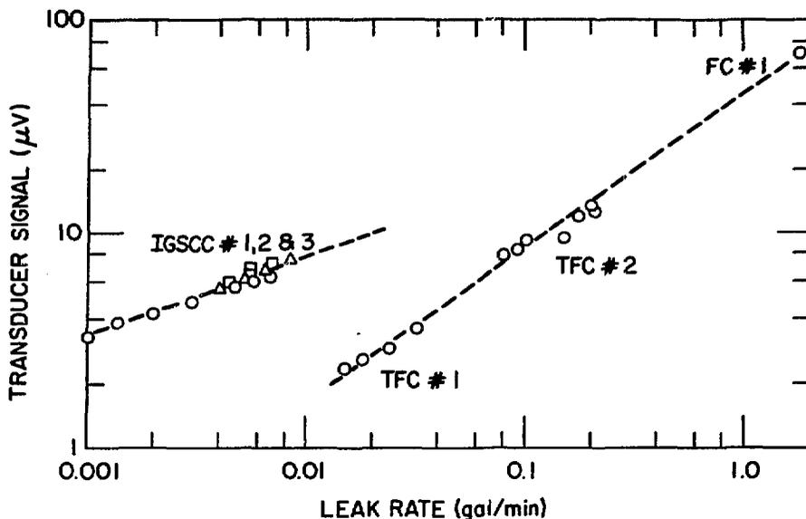
Figure 2. Acoustic Leak Data from Six Cracks Examined at Argonne National Laboratory. Data are normalized as described in the text. Signal amplitudes are for a 300-400 kHz bandwidth after electronic background noise is subtracted.
