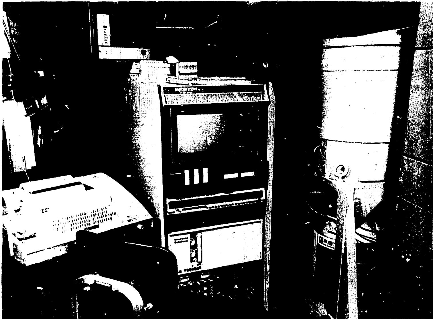
Fig. II-2. Computer based multichannel analyzer and one of three Ge(Li) counting systems.
