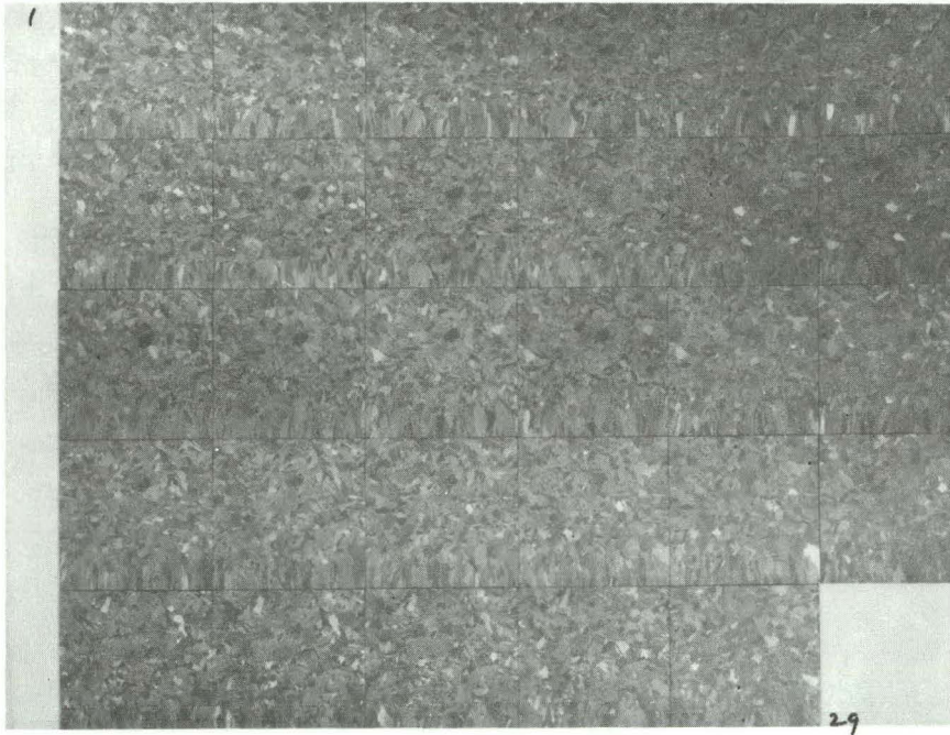
Figure 1 Twenty-nine slices (5 cm x 5 cm) of Wacker SILSO polycrystalline silicon correlated by grain-pattern comparisons at Westinghouse
