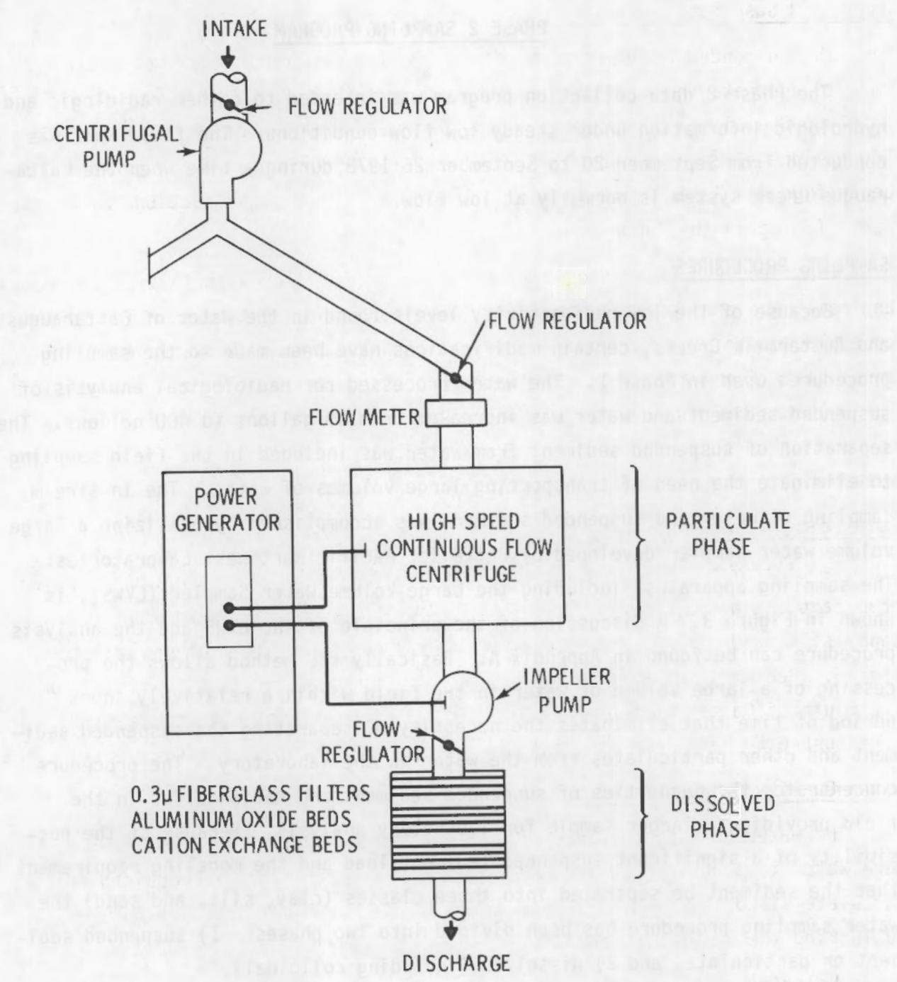
**FIGURE 3.** Phase 2 Sampling Apparatus
