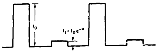
Fig. III-5(a). Chopped pulse train from cw probe laser before the power amplifier is pumped. The chopper wheel has four holes, two of which are open and two of which are covered by \text{CaF}_2 or Mylar attenuators. The attenuation a ranges from about 3 to 6.5.
