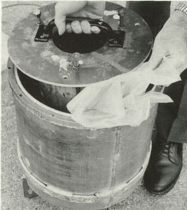
FIGURE 10-29 - Polyethylene after thermal test, configuration-3. The polyethylene sheet located next to the inner container wall stuck together somewhat, but was easily separated.
