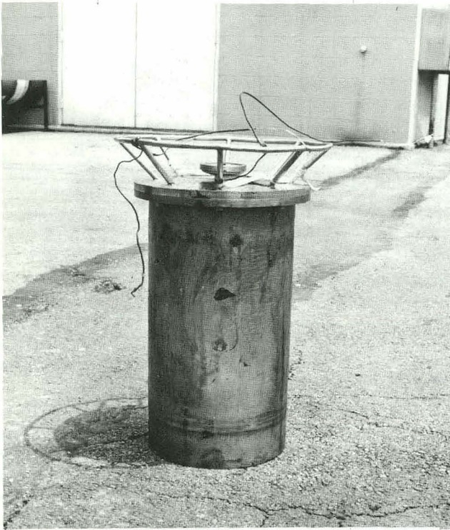
FIGURE 10-26 - Thermal test temperature, configuration-1. The 500°F (260°C) spot of temperature sensitive paint on the side of the inner container did not melt.
