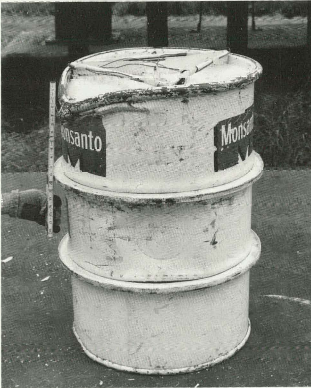
FIGURE 10-19 - After drop and puncture, configuration-1. The dent at the top left resulted from the 30 ft drop and the circular dent at the center resulted from the puncture test.
