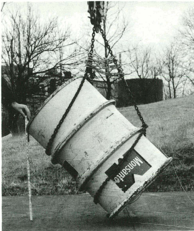
FIGURE 10-5 - Free drop test angle, configuration-1. The container was oriented upside down at a 45° angle to obtain maximum damage.
