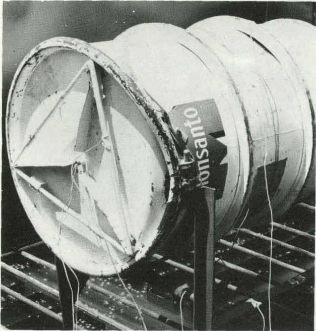
FIGURE 10-10 - Thermal test set-up, configuration-1 with thermocouple attached.
