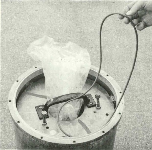
FIGURE 10-28 - O-ring undamaged in thermal test, configuration-3. The silicone O-ring remained "like new" and the polyethylene sheet packaged inside was not damaged.
