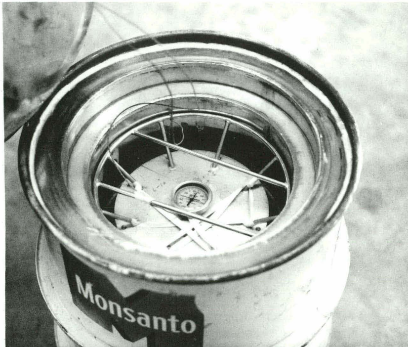
FIGURE 10-1 - Package assembly, configuration-1. Temperature sensitive paints and thermocouples were used. The void between the inner container and the drum assembly is frequently packed with ice during shipment.
