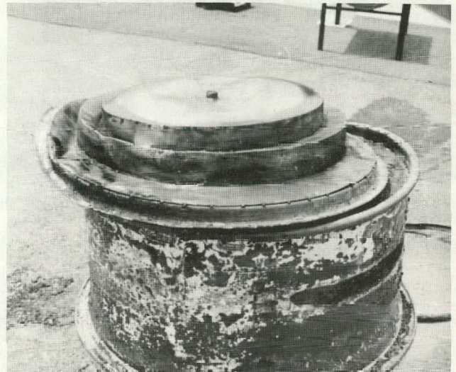
FIGURE 10-21 - Free drop damage to lid, configuration-1.
