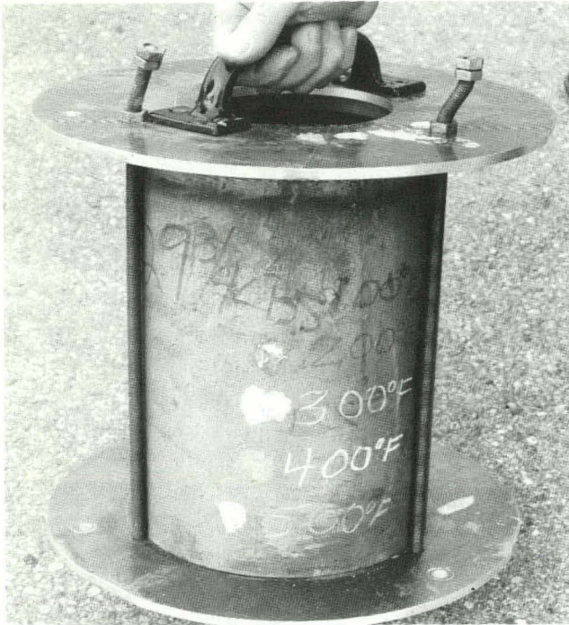
FIGURE 10-30 - Thermal test contents temperature, configuration-3. Temperature sensitive paint indicated that the temperature did not exceed 300°F (149°C). The 200°F (93°C) paint is only partially melted.
