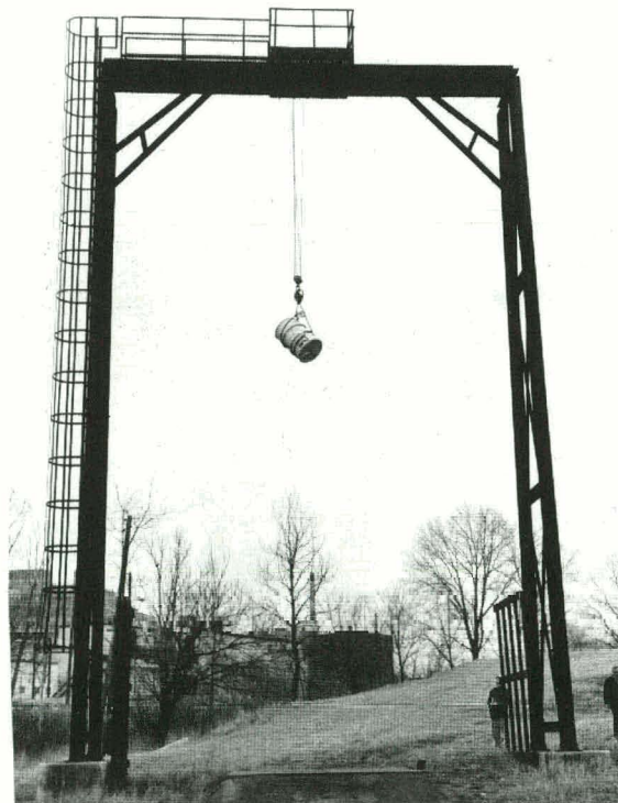
FIGURE 10-6 - Free drop test height, configuration-1. The container is seen suspended at the required 30 ft height.
