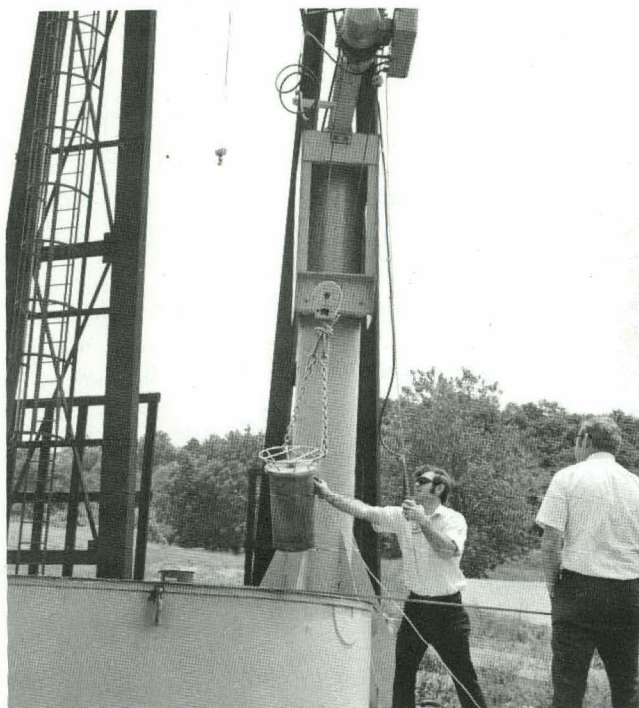
FIGURE 10-16 - Water immersion test equipment, configuration-1. The container is easily lowered into the immersion tank.
