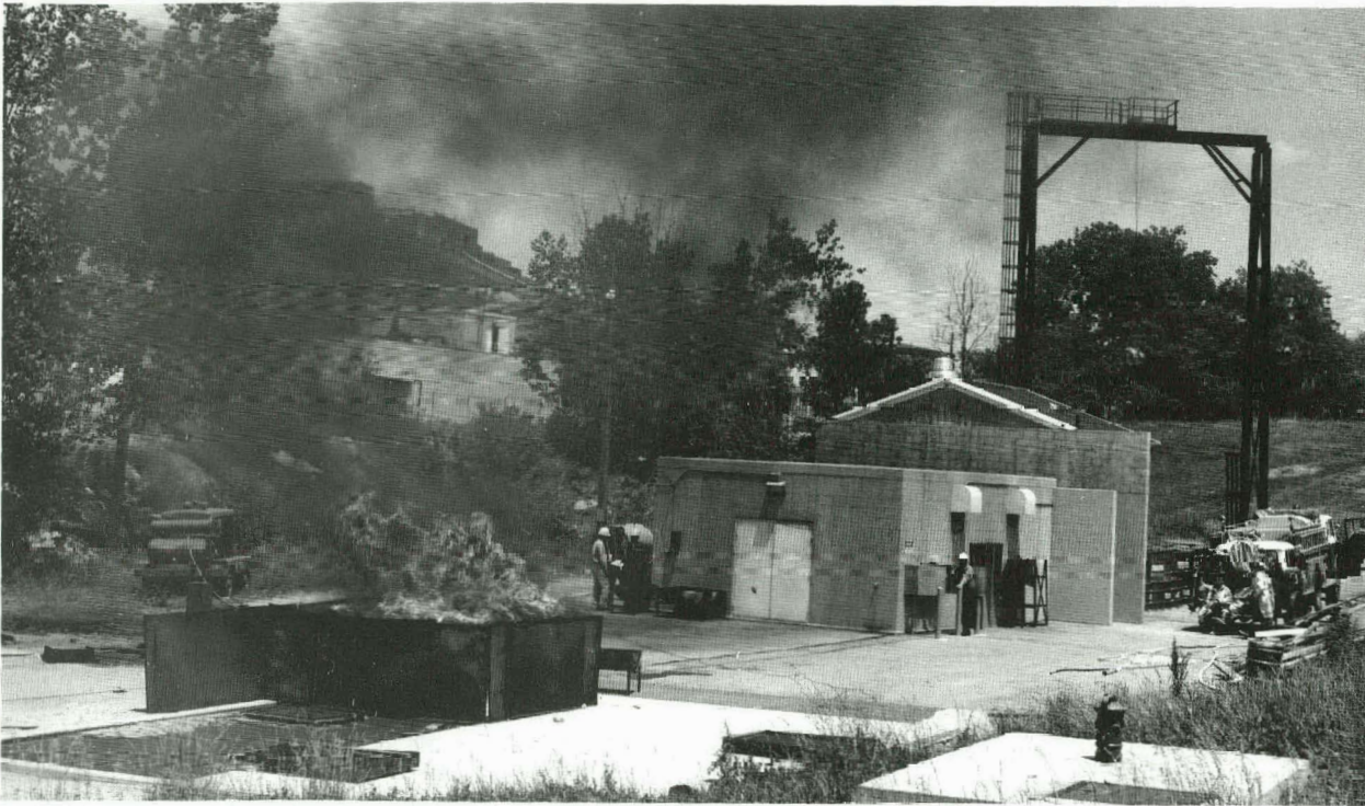
FIGURE 10-11 - Thermal test area, configuration-1 test. The air compressor can be seen in the left background and the temperature recorder in the center background. The fuel flow was controlled at the panel mounted on the outside wall of the concrete block building as seen at the right. Firemen and firefighting equipment are at the far right.
